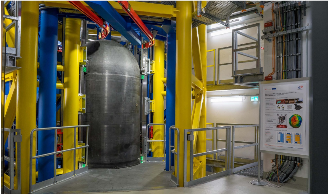
Figure 1. Start position of the Einstein-Elevator gondola for a vertical parabolic flight (credit: Leibniz University Hannover/Marie-Luise Kolb, licence: CC-BY 3.0 DE ).
