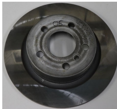
Fig. 3. Tungsten carbide-coated brake disc of the BMW i3
