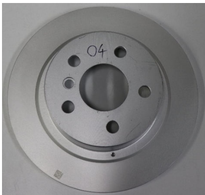
Fig. 2. Original cast iron brake disc of the BMW i3
