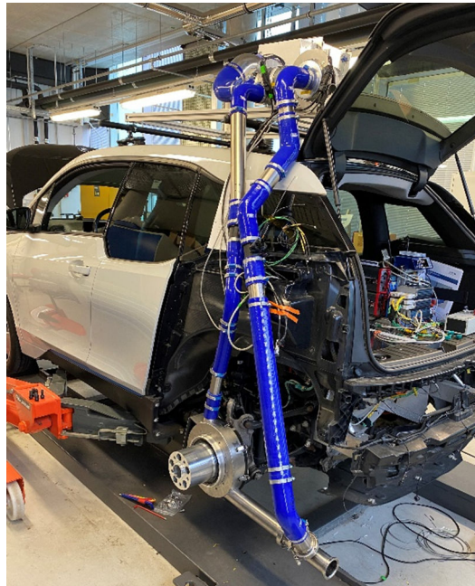
Fig. 8. Enclosure and ventilation system of the brake on the reference test vehicle
