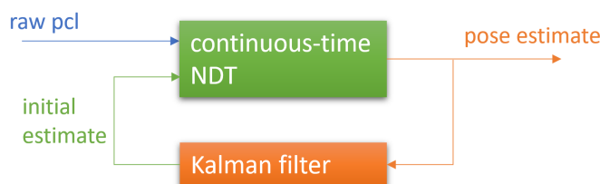
Figure 4. Feedback loop when using the continuous-time NDT formulation and the filter prediction as an initial estimate of the tracking result.
