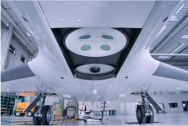
Figure 6: LDA sensor plate mounted in the front lower viewport with 4 apertures.
