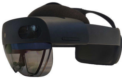
Figure 2: The Microsoft HoloLens 2 can track the user's hands and eyes to enable a variety of interaction possibilities.
