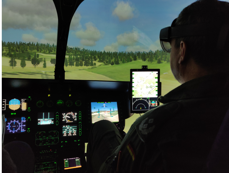
Figure 1: A pilot sits inside DLR's helicopter simulator AVES using the Microsoft HoloLens 2 as a see-through HMD. A synthetic vision system in front, a topographical map, a Navigation Display and a Primary Flight Display to the left provide additional information.
