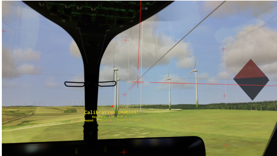
Figure 3: A wireframe box is used to calibrate the HoloLens view with the dome projection of the AVES helicopter simulator. In red the wireframe as it would be rendered on the HoloLens is shown. The white equivalent is part of the dome projection. The octahedron at the far right of the image represents the simulator's design eye point position. Here, an uncalibrated state is shown for demonstration purposes.
