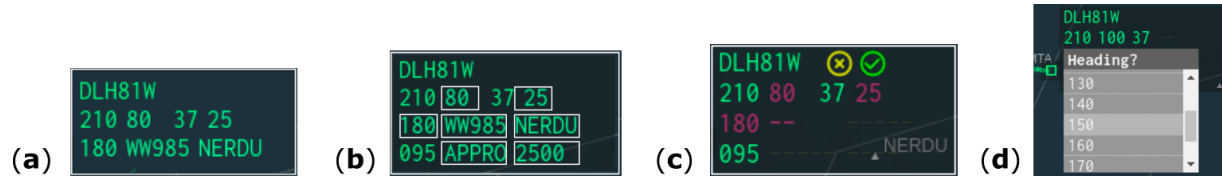
Figure 4. (a) Reduced (standard) aircraft data block, (b) full aircraft data block, (c) full aircraft data block with ASRU output, (d) drop-down menu to manipulate radar label cells.
