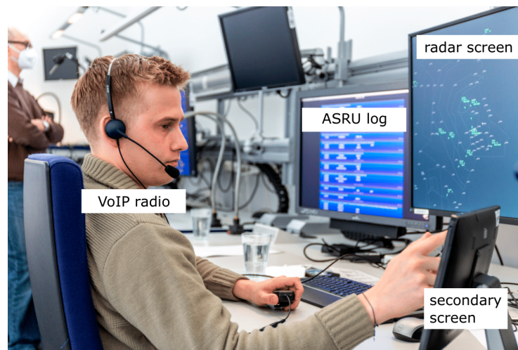
Figure 1. CWP setup including headset for radio telephony, radar screen, ASRU log, and secondary screen.
