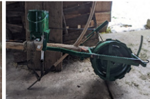
A direct planter prototype from Tanzania. The idea was to make the planter as low-cost as possible. In theory, this planter could be used through cover crops.
