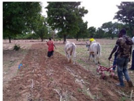
Weeder in action; it can also be used as skim plough with a 3-times higher area performance and a much lower draft necessary draft than a traditional plough (Photo: Robert Burdick)
