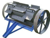
Animal drawn knife roller in transport position with staggered and increased numbers of knives. (Photo: Saidi Mkomwa)
