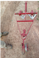
Weeder from Burkina Faso with three sweeps with low angle low crown for shallow weeding (Photo: Robert Burdick)
