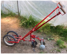
A hand-held weeder with protective discs, as used for row crops by small farms in Europe. (Photo: FiBL)
