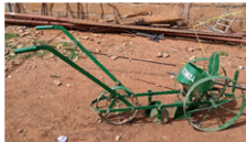
Planter prototype from Burkina Faso designed for use in fields with or without residue.
