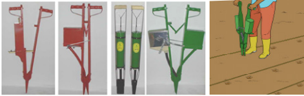
Different types of jab planters, without fertiliser hoppers (left) and with fertiliser hoppers (right)
