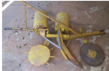
Direct injection planter with fertiliser hopper as used in Southern Africa. The front coulter cuts through a cover crop to allow the planter easy access. The back drive wheel serves to turn the seed plates.
