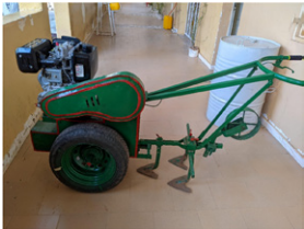
A two-wheeled tractor with weeding sweeps from Senegal. (Photo: Robert Burdick)
