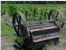
Animal-drawn knife roller in working position. In this type, the metal blades are welded to a metal ring fitted on a solid wooden trunk, with wheels attached for easy transport to the field. (Photo: Saidi Mkomwa)
