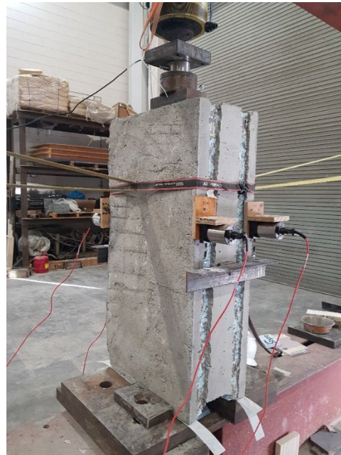
Fig. 11 Double shear specimen test setup
