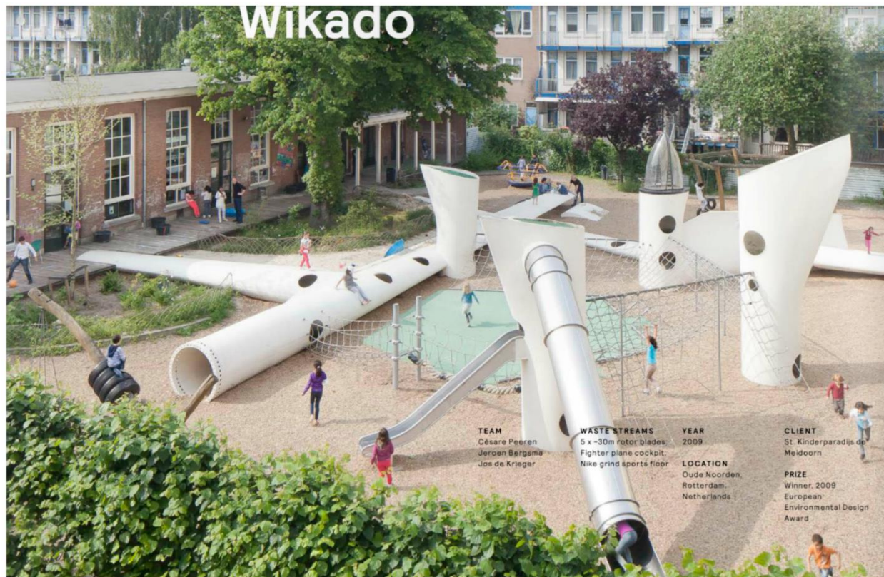
Figure 2. Example of wind turbine blades being repurposed. These blades were reused as materials for a playground constructed in 2009 in the Netherlands (Mishnaevsky et al., 2017).
