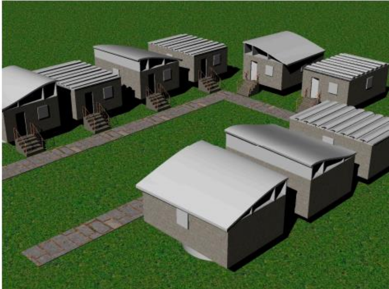
Figure 11. Rendering of affordable housing built using parts of wind turbine blades (Bank et al., 2018).
