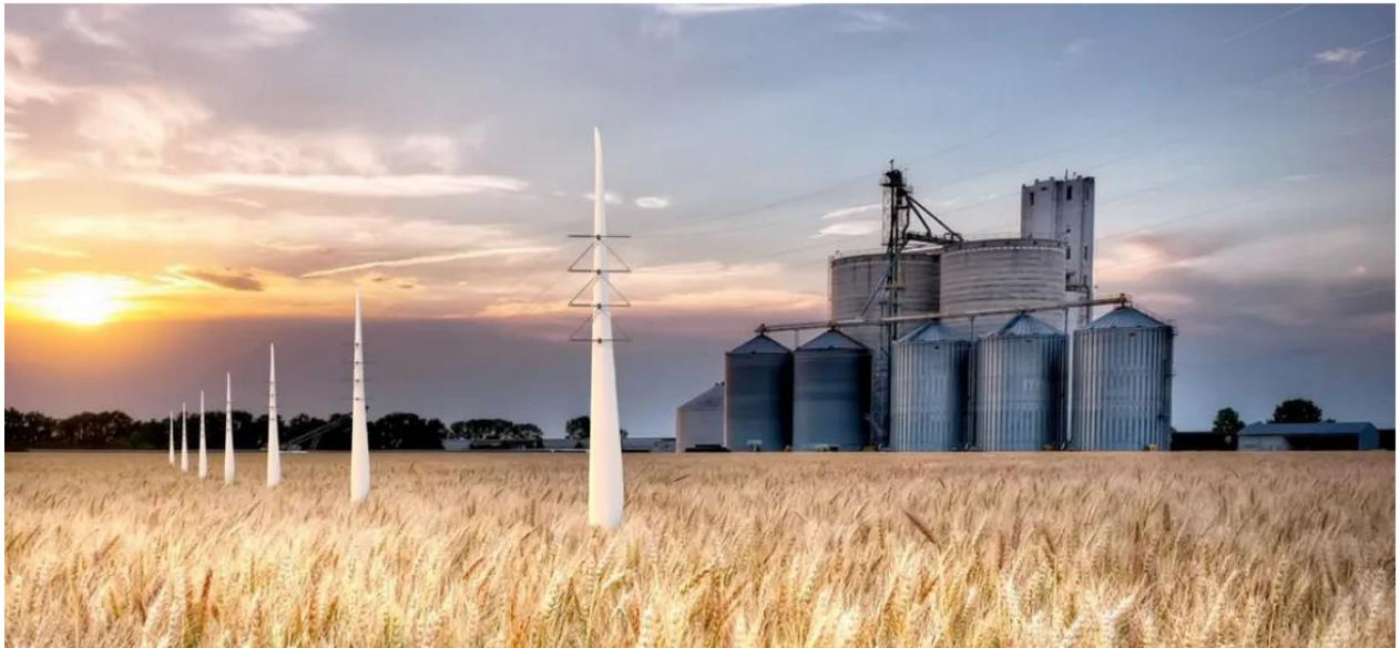
Figure 10. Rendering of wind turbine blades being used as utility poles as part of the BladePole project in Kansas (Gallucci, 2022).
