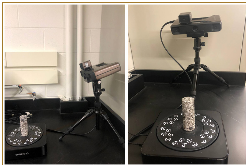
Test set up for determining the bulk specific gravity of compacted asphalt mixture specimens
