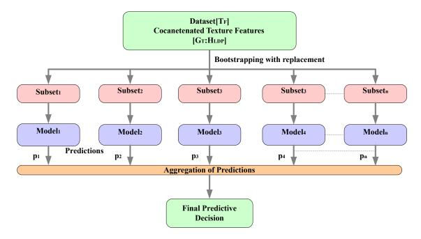
Fig. 5: Framework of Bagging ensemble method.
