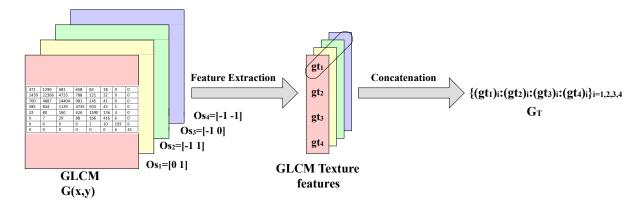
Fig. 3: Texture feature extraction from GLCM.
