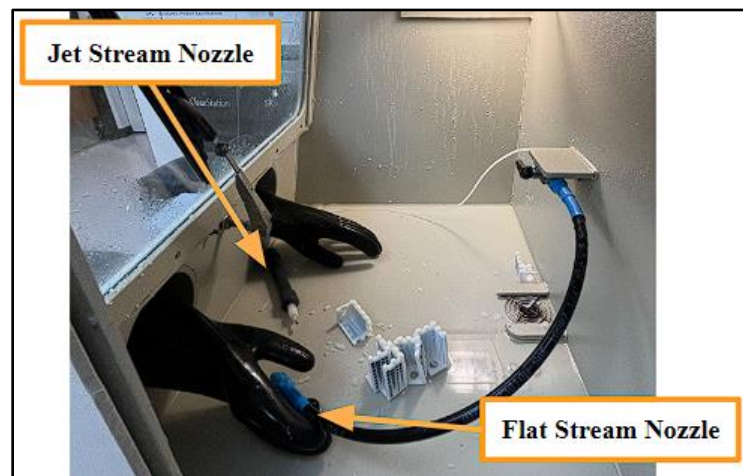
Figure 37: The water jet cleaning station for post-processing PolyJet parts is a small glovebox with hoses for different nozzle attachments.
