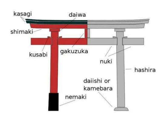
A Torii is a Japanese Gate structure used to signify a place of importance. It consists of two posts called Hashiras, a middle beam called the Nuki, and two top beams called the Kasagi and Shimaki.
