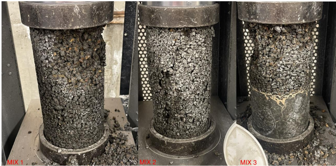
Figure 2. Examples of Concrete Samples prior to Compression Testing
