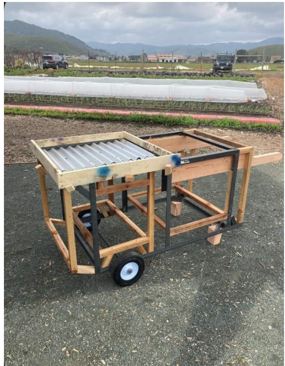
Figure 5: Finished Framing/ Ready for Casting
