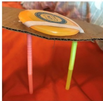
Figure 4. Actuator Extending to Manipulate Anhyzer Angle
