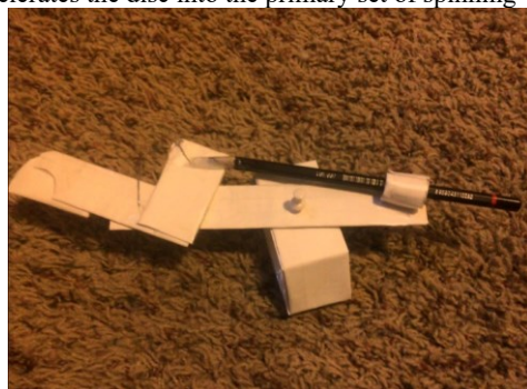
A spinning arm with an actuator positioned to balance the arm. The actuator causes the force in the wrist of the arm.
