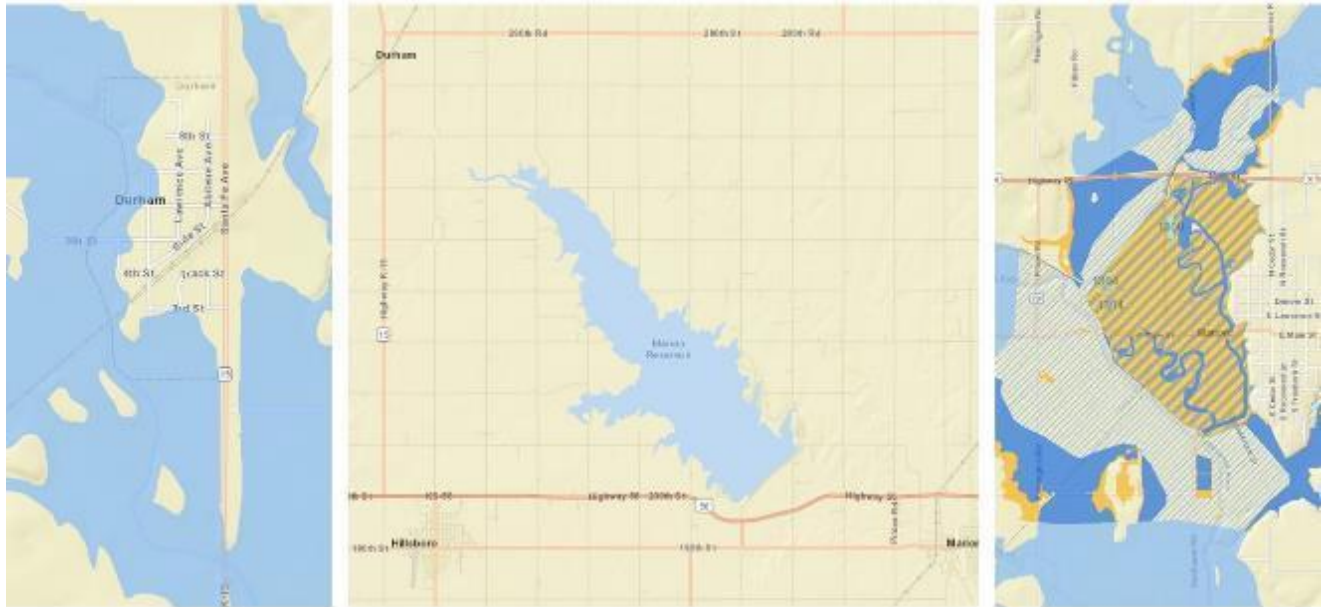
Figure 6.7. Marion Dam (Reservoir) DFIRM illustrates differences in flood information available to the cities of Durham (upstream) and Marion (downstream). Source: KDA Kansas Floodplain Viewer (2021).
