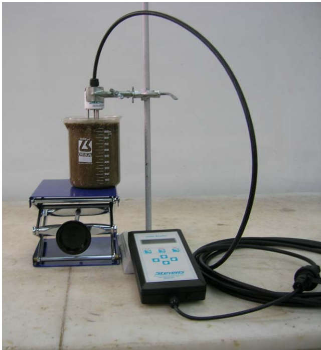
Figure 1. Experimental set-up for dielectric permittivity determination of sand samples with different amounts of fluids using the HydraProbe sensor
