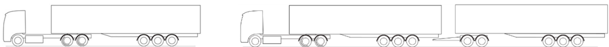
Figure 1. Tractor and semitrailer (prototype) with the nominal GVW 40 tonnes configuration (left) and a HCT configuration of tractor, semitrailer, dolly, and another semitrailer with GVW of 76 tonnes (right).
