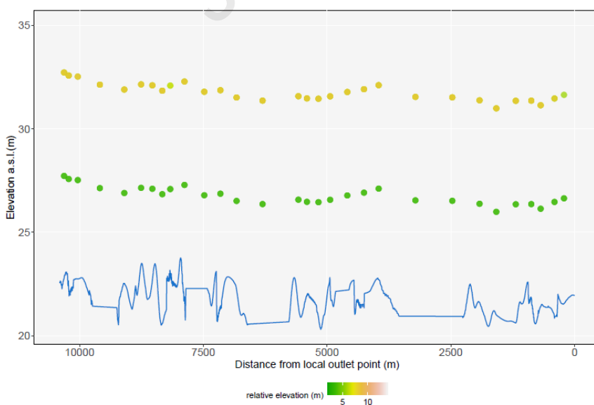
Fig. 4— Terrace-like surfaces along with the longitudinal profile of the NSR watercourse in the Manucho stretch, applying the script by Jodza (2019). The extraction of relative elevations from discrete terrace levels
