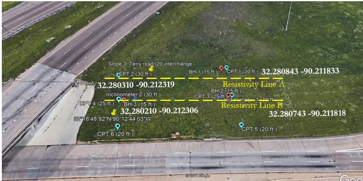
Figure 4.17 Location of Slope 3 and ERI Test Lines
