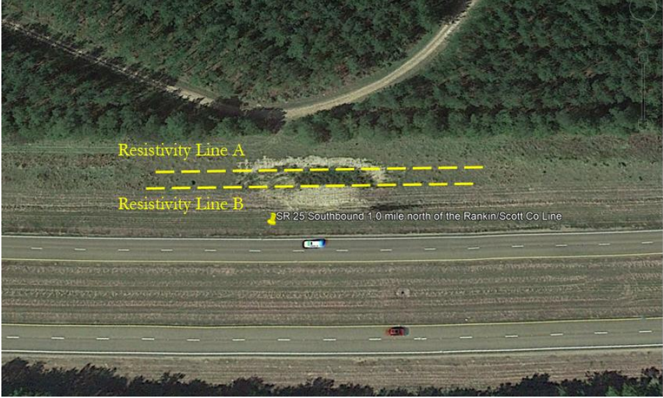
Figure 4.56 ERI Location in Failed Slope 3
