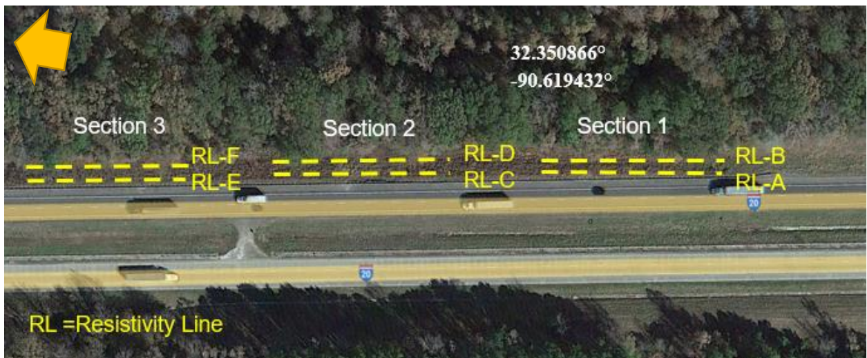
Figure 4.68 Location of ERI Test Lines in Failed Slope 5 (Big Black River)
