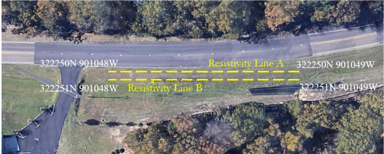
Figure 4.116 Location of ERI Test Lines in Failed Slope 19
