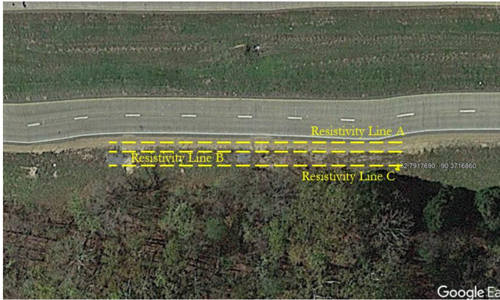
Figure 4.90 Location of ERI Test Lines in Failed Slope 10
