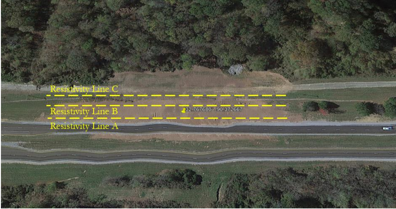
Figure 4.81 Location of ERT Test Lines for Failed Slope 7
