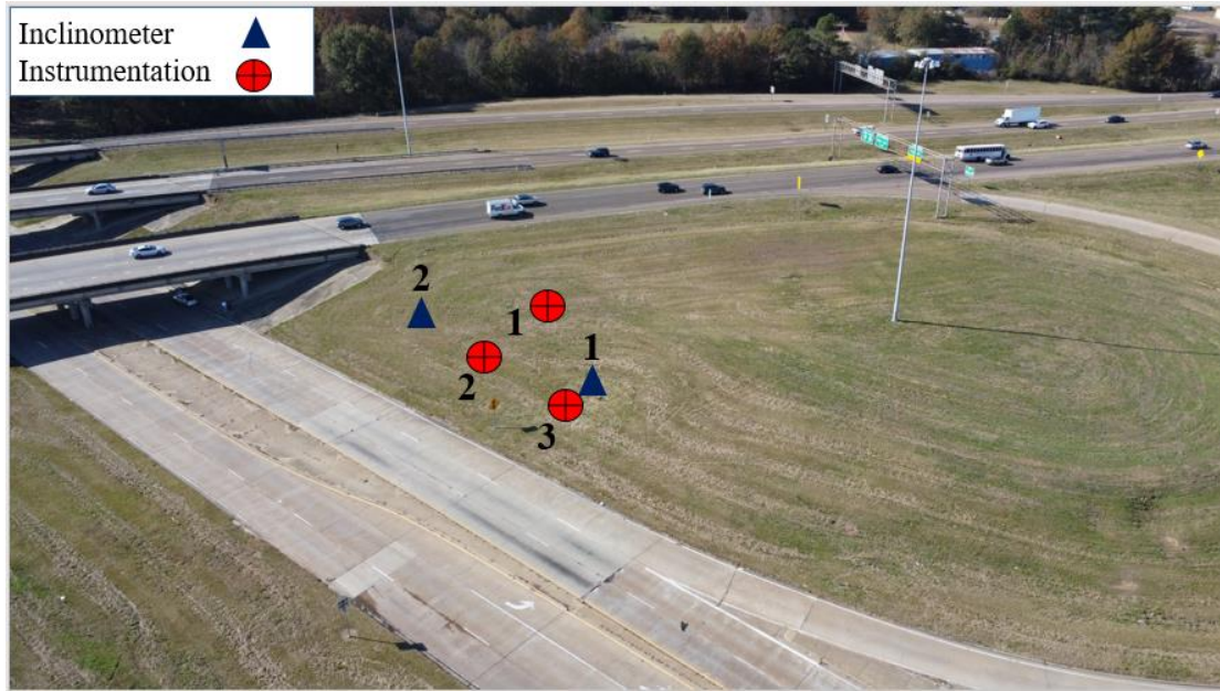
Figure 3.24 Instrumentation Layout at I-Slope 3
