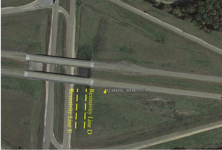
Figure 4.60 Location of ERI Lines at Failed Slope 4 - SR25/43 Interchange Left Abutment
