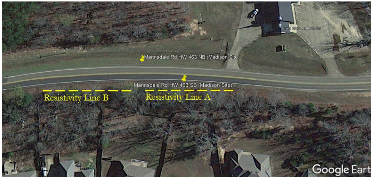
Figure 4.121: ERI Test Lines at Failed Slope 20
