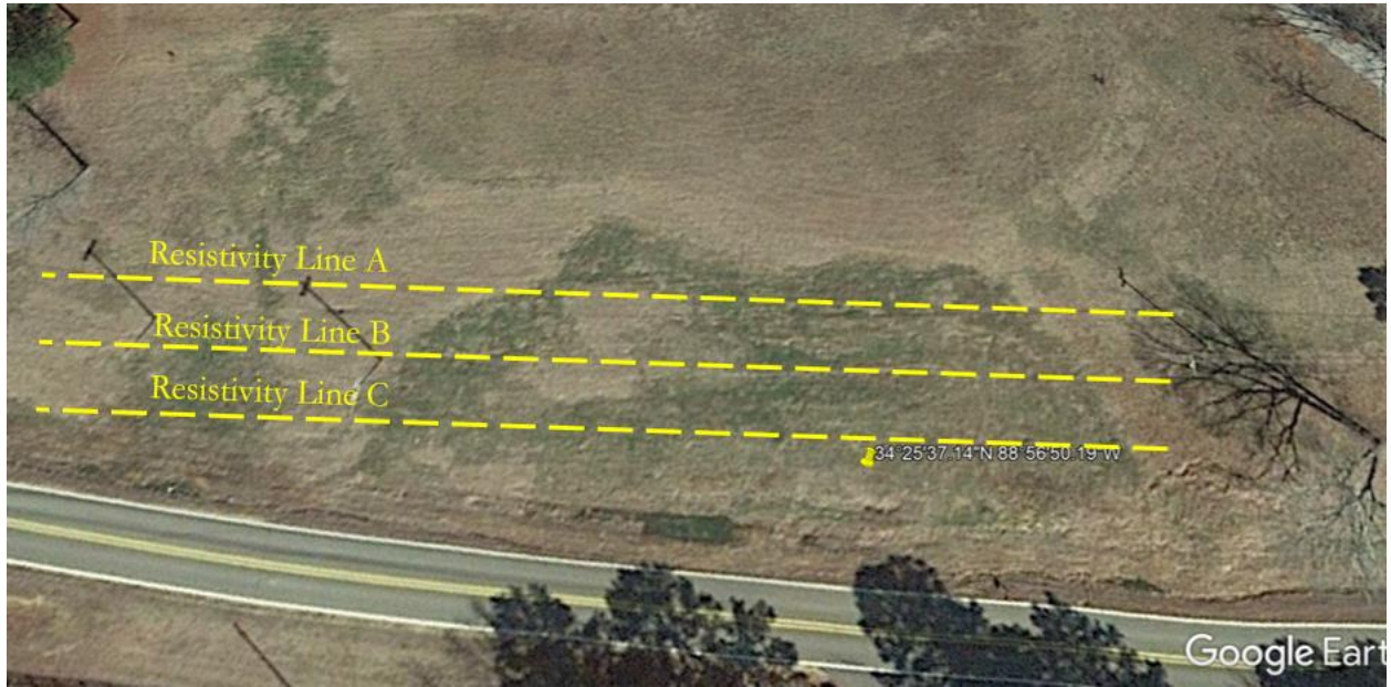
Figure 4.84 Location of ERI Test Lines in Failed Slope 8
