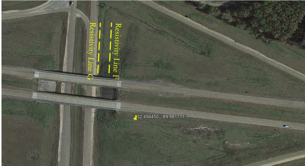
Figure 4.62 ERI Test Location of Failed Slope 4- SR25/43 Interchange Right Abutment
