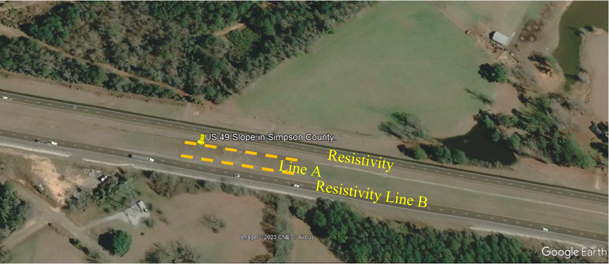
Figure 4.98 Location of ERI Test Lines in Failed Slope 14
