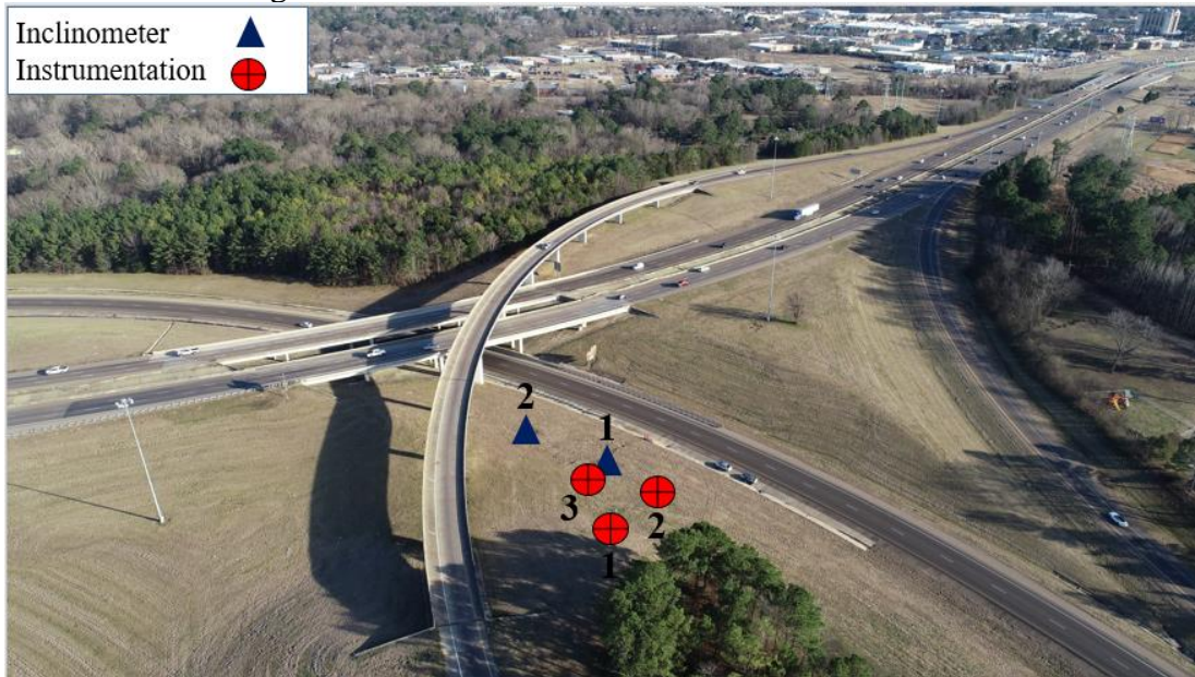
Figure 3.4 Instrumentation Layout at I-Slope 1
