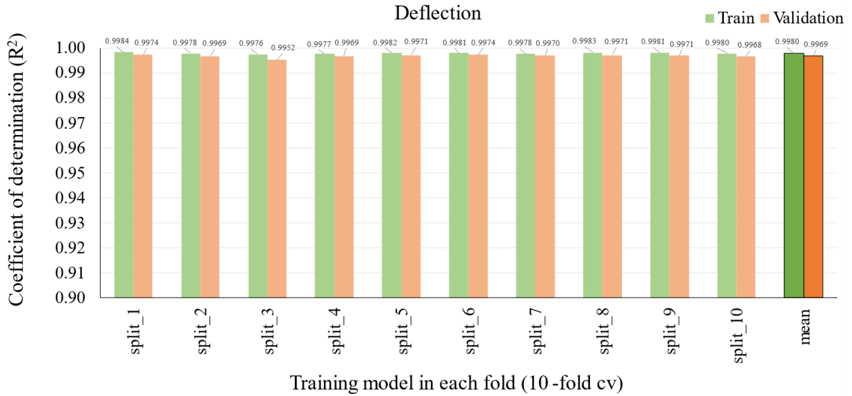
Figure 42. Accuracies of training and validation data sets for pavement systems with stabilized and granular bases
