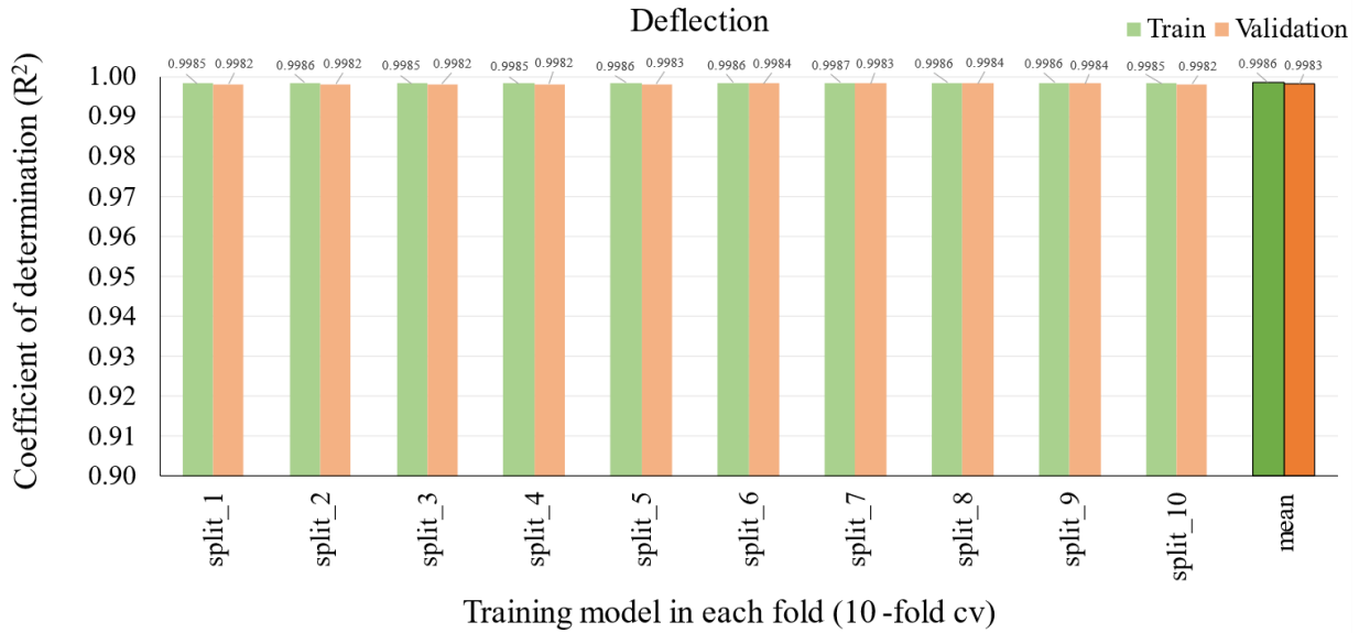
Figure 34. Accuracies of training and validation data sets for pavement systems with a granular base
