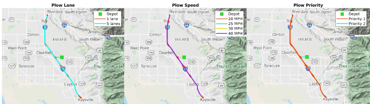
Figure 3.8 Plowing lanes, travel speed and road priorities along I-15 in group 1 within Clearfield
