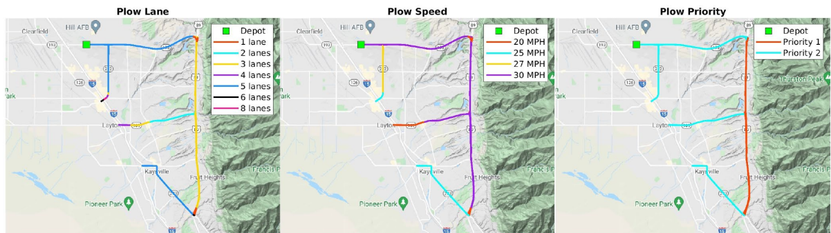
Figure 3.11 Plowing lanes, travel speed and road priorities along SR-109, SR-232 and SR-273 in group 4 within Clearfield
