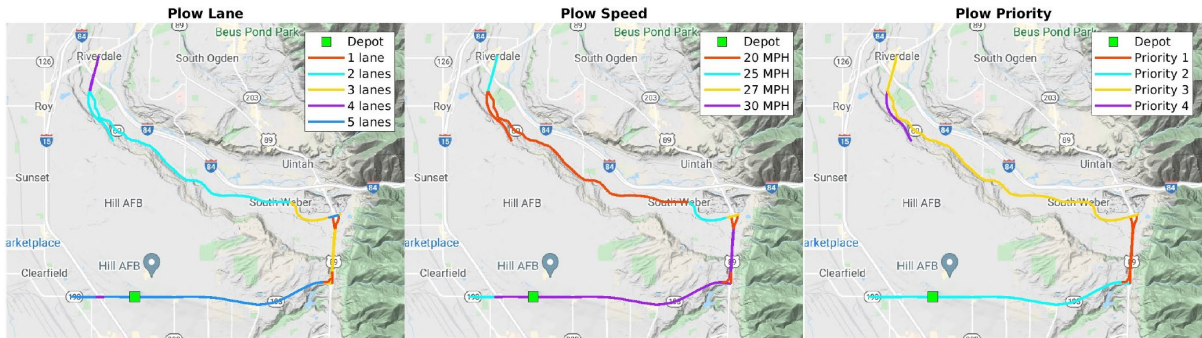
Figure 3.10 Plowing lanes, travel speed and road priorities along SR-193, SR-60 and SR-168 in group 3 within Clearfield
