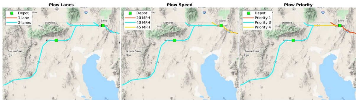
Figure 5.1 Plowing Lanes, travel speed, road priorities within Snowville
