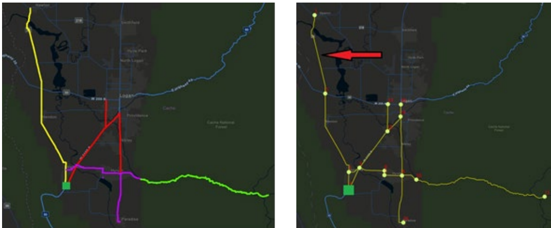
Figure 2.1 The planned roadways (left) and resulting network edited in ArcGIS pro (right). The green box represents the maintenance station (also referred to as the depot).
