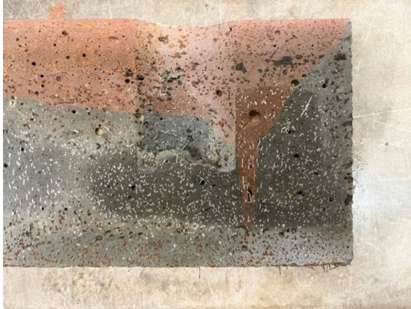
Figure 101: Cut prism shows interface deformation due to rodding
