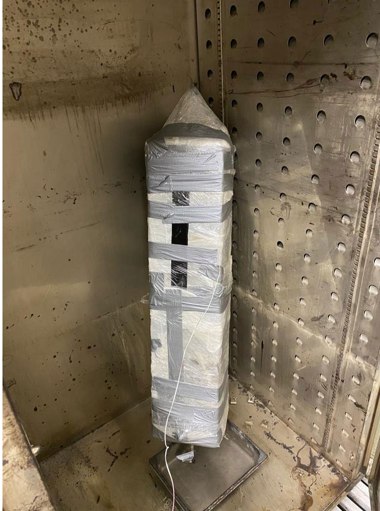
Figure 197: Column specimen during steam curing
