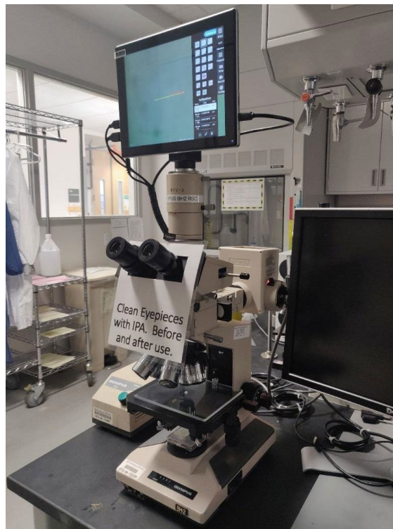
Figure 238: The microscope that was used to scan and determine the thickness of the steel fibers, the microscope is attached with a tablet computer to digitally measure and record the thickness of the steel fibers
