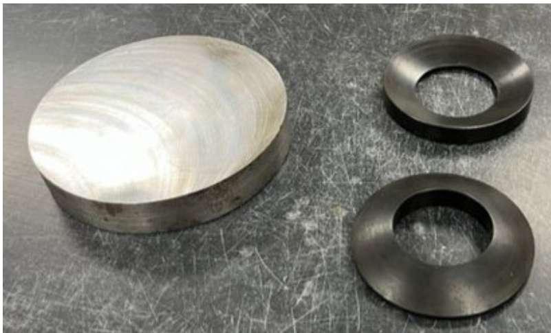
Figure 107: Milled steel platen and spherical washer
