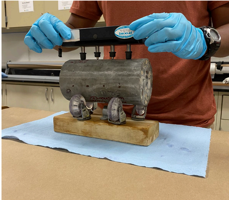
Figure 152: Surface resistivity test set up
