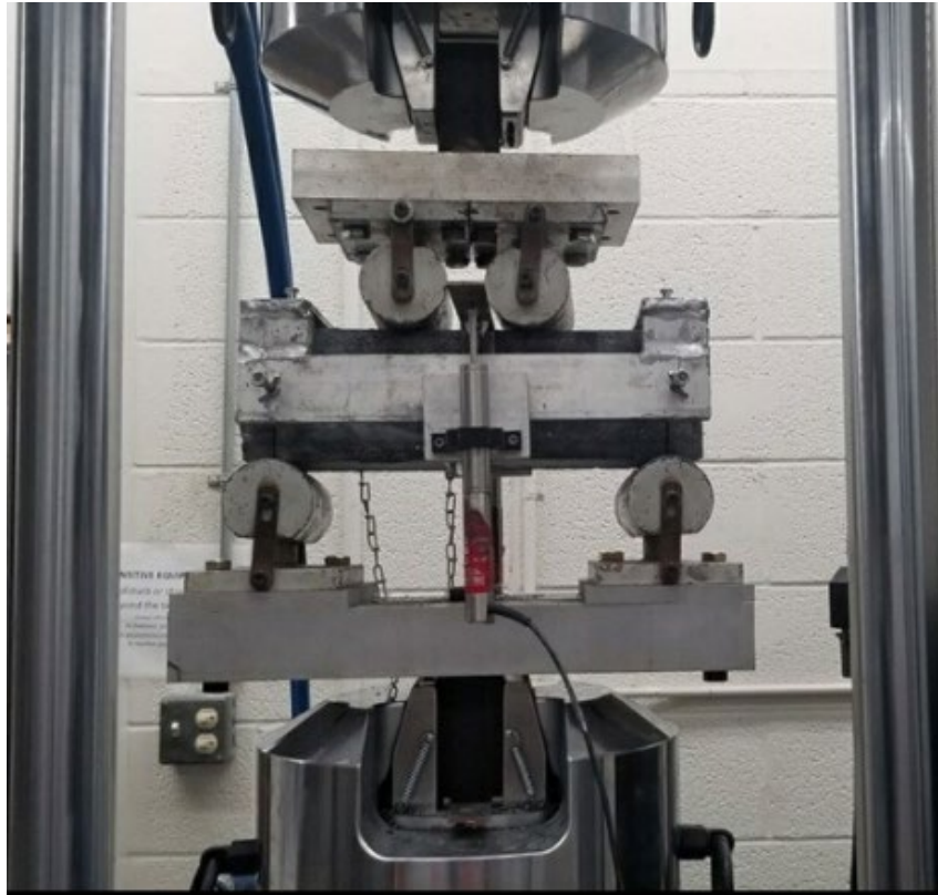
Figure 6: Sample at University of Florida during testing according to ASTM C1609
