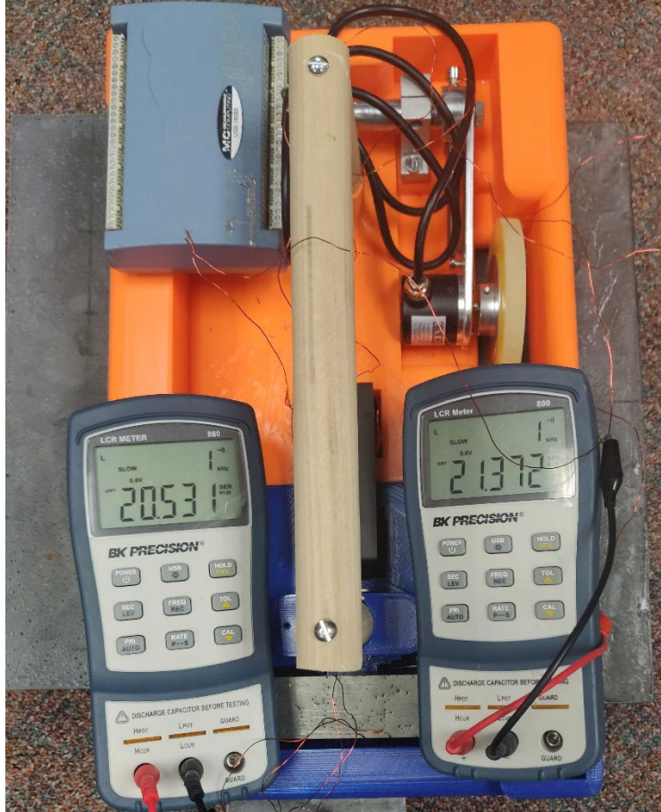
Figure 212: Third prototype with two electromagnets, LCR meter, encoder for location measurement, and data acquisition system, all enclosed in a 3D printed case with a wooden handle and wheels
