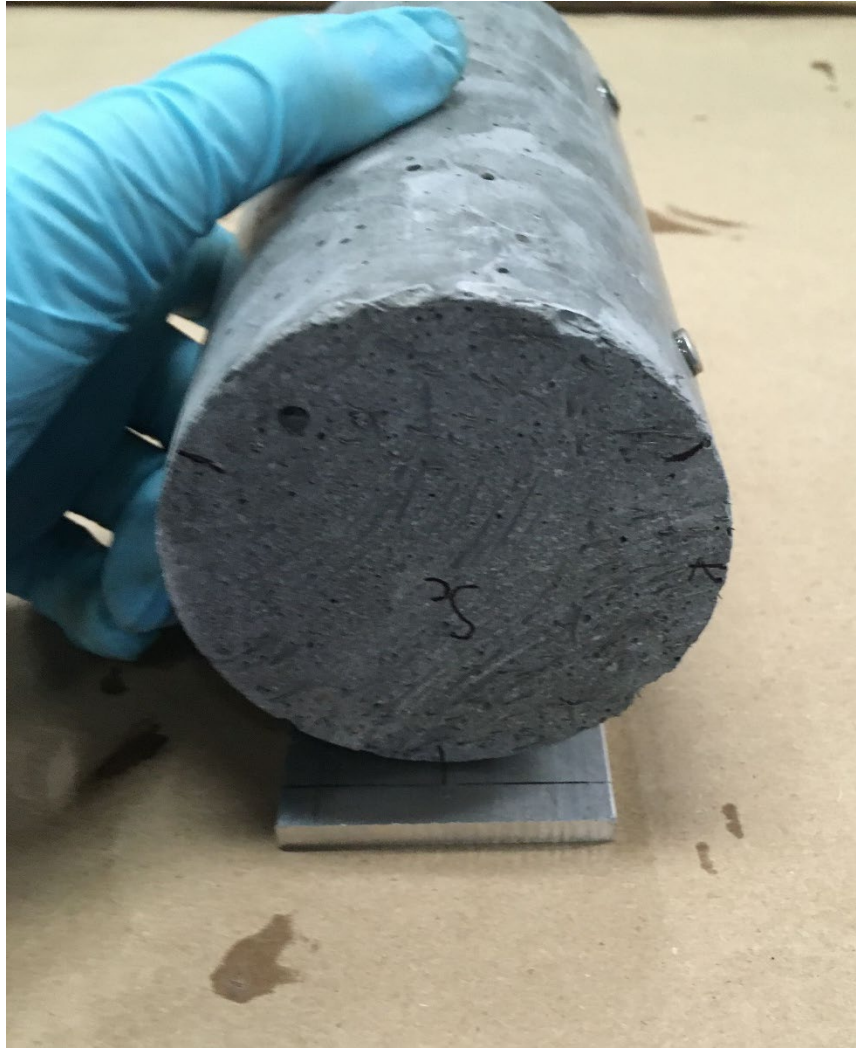
Figure 106: Cylinder is lined up on template to adhere gauge points
