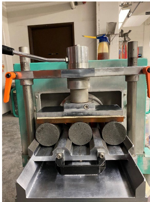
Figure 151: Grinding UHPC samples for resistivity measurements
