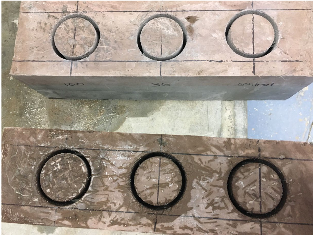
Figure 82: Cores in layered prisms
