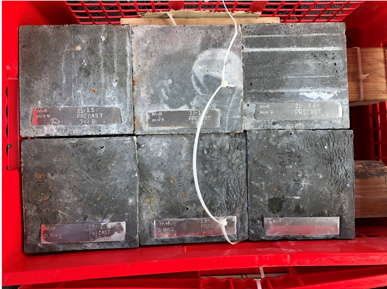
Figure 198: Concrete cube samples with labels
