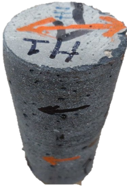
Figure 223: Picture of the core with markings made before taking it out (orange double-headed arrow) and the ones made right after taking the cores (single-headed black and orange arrows)
