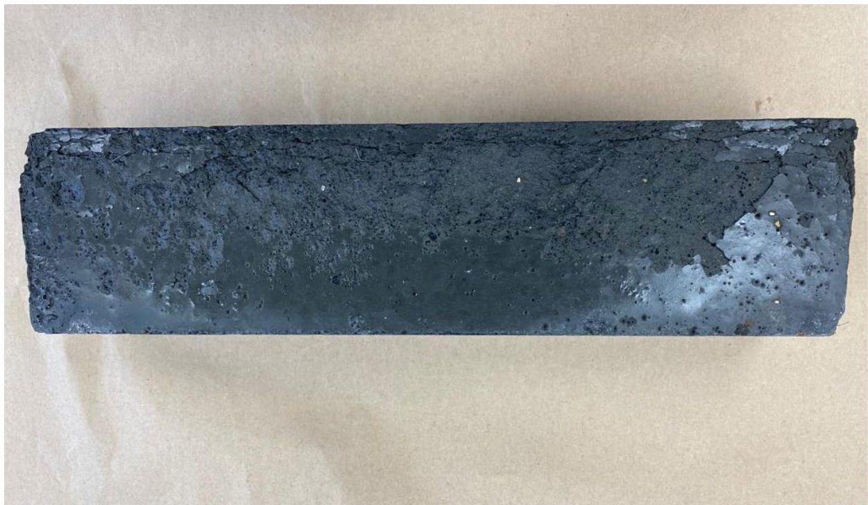
Figure 130: photo of the 12 ksi steam-cured specimen after 330 cycles
