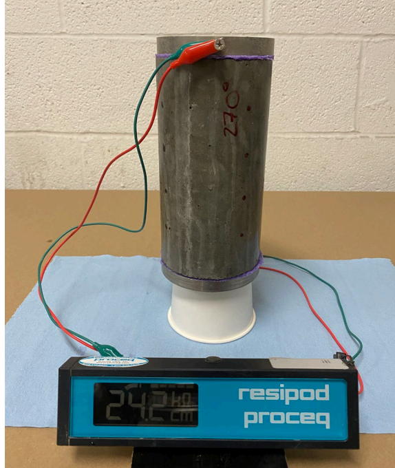
Figure 153: Bulk resistivity test set up
