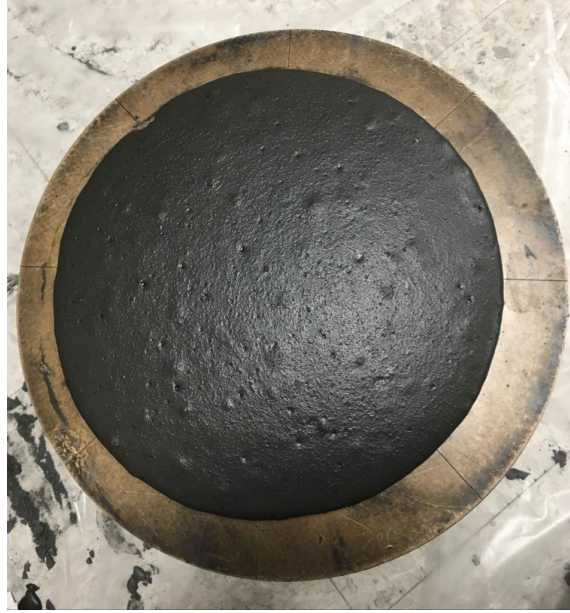
Figure 3: Static flow test with measurement of ~8.5 in
