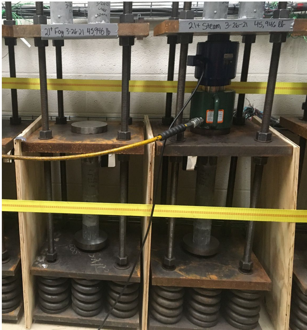
Figure 108: Two creep frames, one being loaded with hydraulic jack
