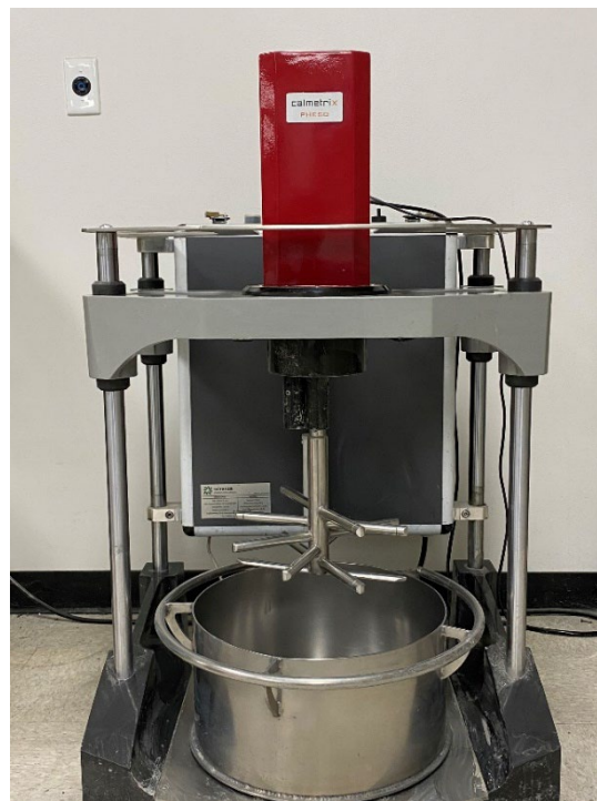
Figure 147: Pheso Rheometer mixer for UHPC batches up to 0.13 ft 3
