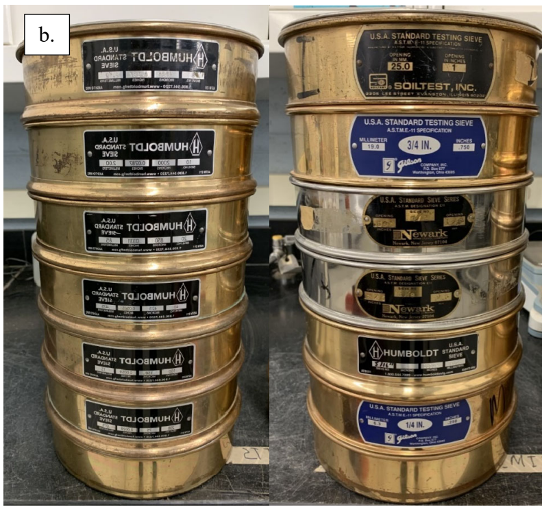
Figure 3.3 Equipment used for gradation analysis: (a) sieve shaker (b) sieve stacks (Morro 2021).
