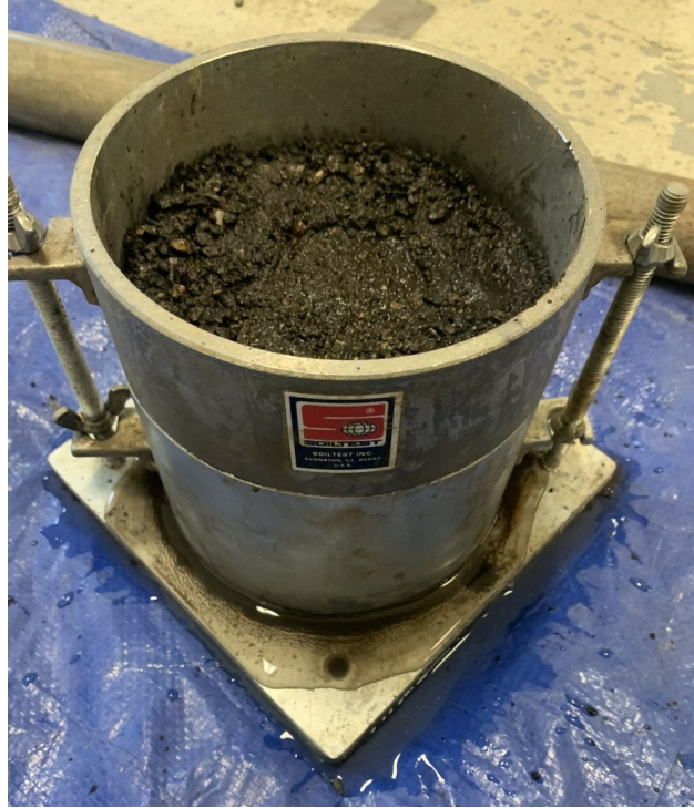
Figure 3.21 RAP compacted wet of optimum (Morro 2021).
