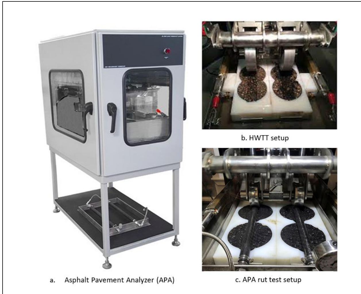
Figure 29. APA and HWTT Rutting Test in the Asphalt Pavement Analyzer
