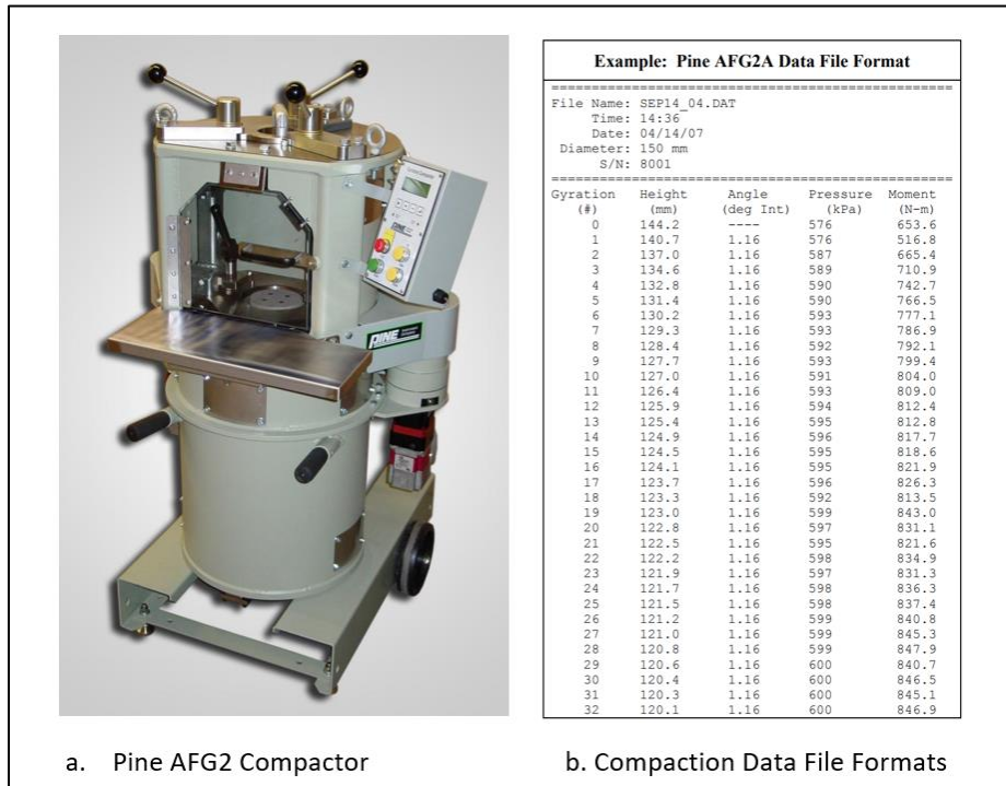
Figure 33. the Pine Superpave AFG2 Gyrotory Compactor (SGC)
