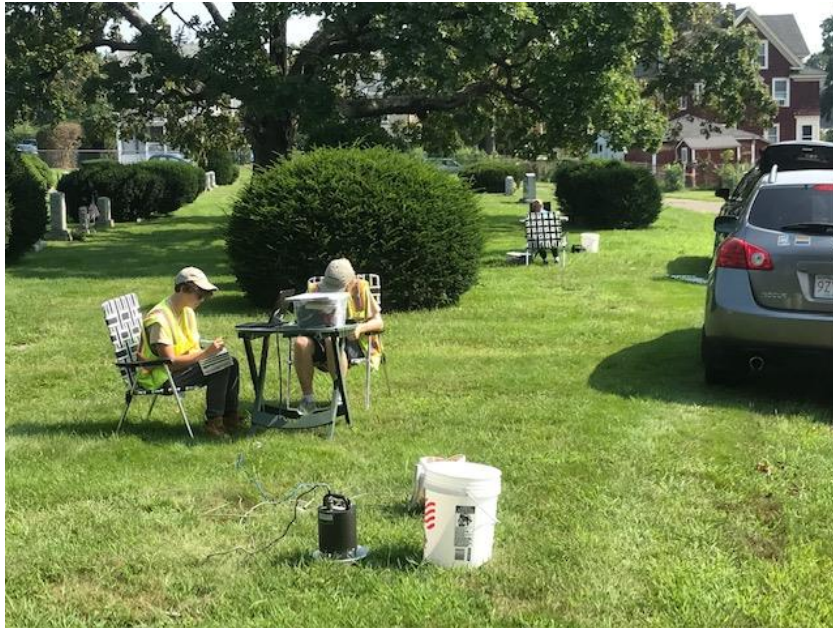
Figure 2.1: Students collecting HVSR survey data in Northampton, MA. Seismometer is the instrument in the foreground
