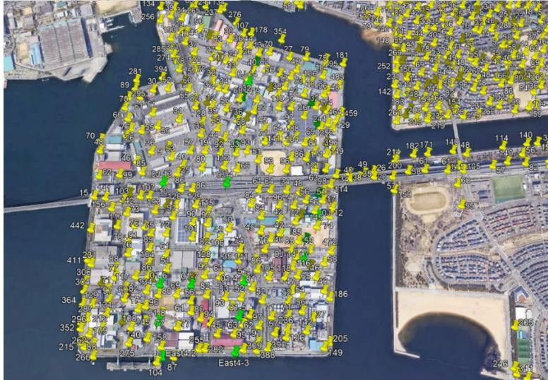
Figure 5.5 Process of borehole location digitization (a) Google maps view of a site in Kobe, Japan, (b) boreholes overlaid and digitized, and (c) displacements (yellow pins) digitized with boreholes (green pins)
