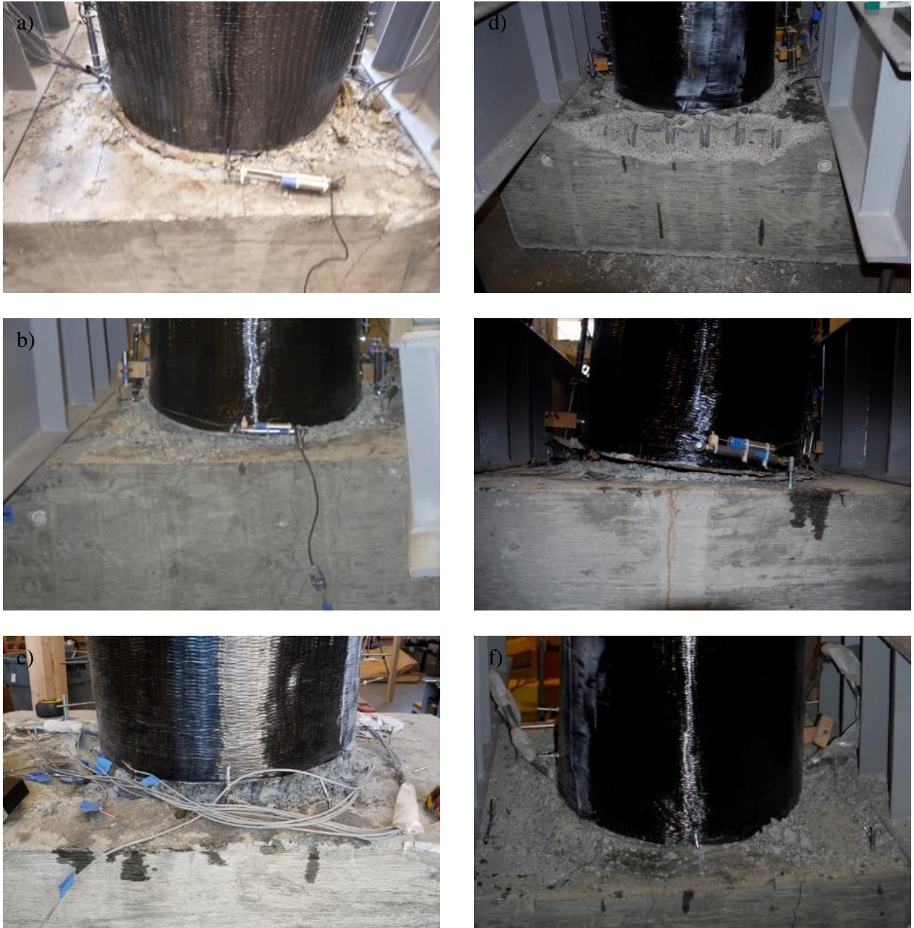
Figure 3.24. Concrete Damage at Base at Completion of Testing for: a) C(CFRP)-4.0-#7(1.3)-0.05, b) C(CFRP)-4.0-#5(1.4)-0.05, c) C(CFRP)-4.0-#7(2.7)-0.05, d) C(CFRP)-4.0-#7(1.3)-0.05-EQ, e) C(CFRP)-4.0-#7(1.3)-0.05-2X, and f) C(CFRP)-4.0-#7(1.3)-0.15
