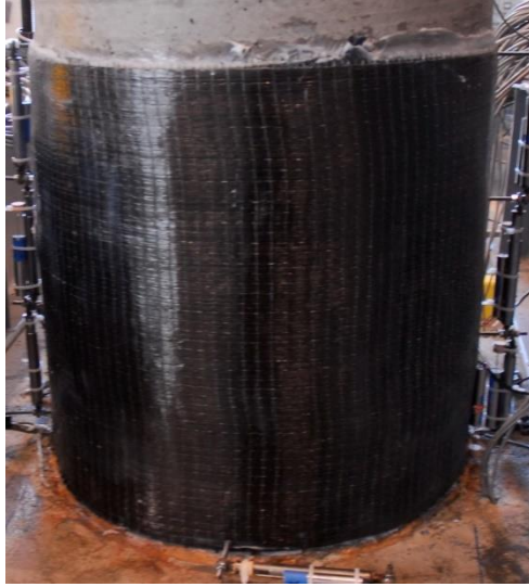
Figure 3.4: CFRP Jacket Before Testing for C(CFRP)-4.0-#7(1.3)-0.05
