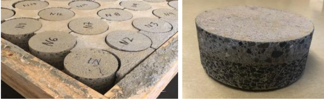
Figure 3.4 Cylindrical sample preparation for the shear and tensile bond strength tests
