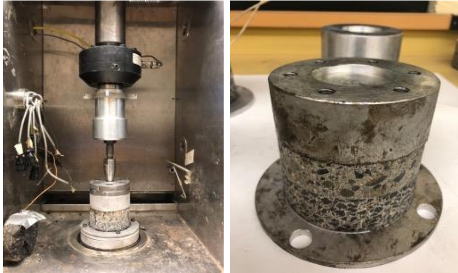
Figure 3.10. Tensile strength test of shotcrete-concrete interface bond
