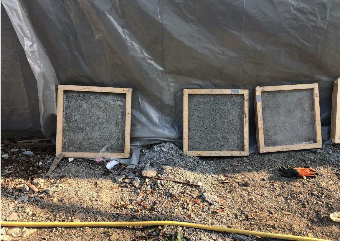
Figure 3.1 Concrete panels for bond strength samples after surface preparations: (left) pressure-washed; (middle) chipped; and (right) sandblasted
