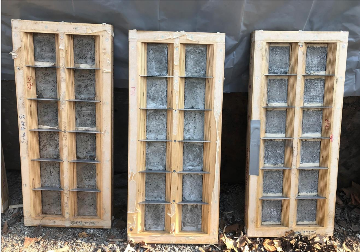
Figure 3.2 Concrete panels for double-wedged samples after surface preparations: (left) sandblasted; (middle) pressure-washed; and (right) chipped
