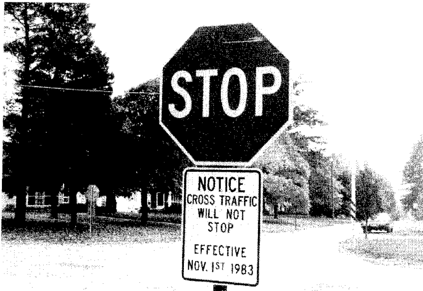
FIGURE 41. NOTICE SIGN BENEATH STOP SIGN ON WARD PARKWAY PLAZA PRIOR TO CONVERSION. (KANSAS CITY, MISSOURI)
