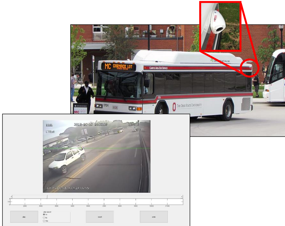
Figure 2.1-1: Driver’s side exterior camera used to record imagery used in empirical studies with sample frame of video imagery shown in project’s Graphical User Interface
