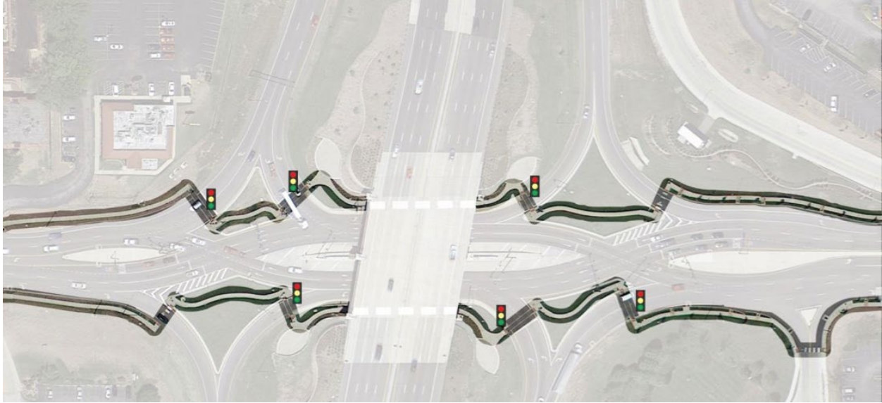
Figure 5.3 Pedestrian Access Outside of a DDI in Maryland Heights, MO [Adapted from (30)]
