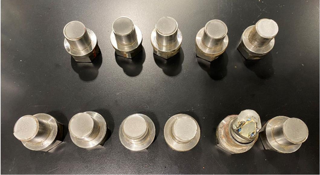
Figure 75. All shear bolts broke cleanly, except #5 (bottom row, second from right)
