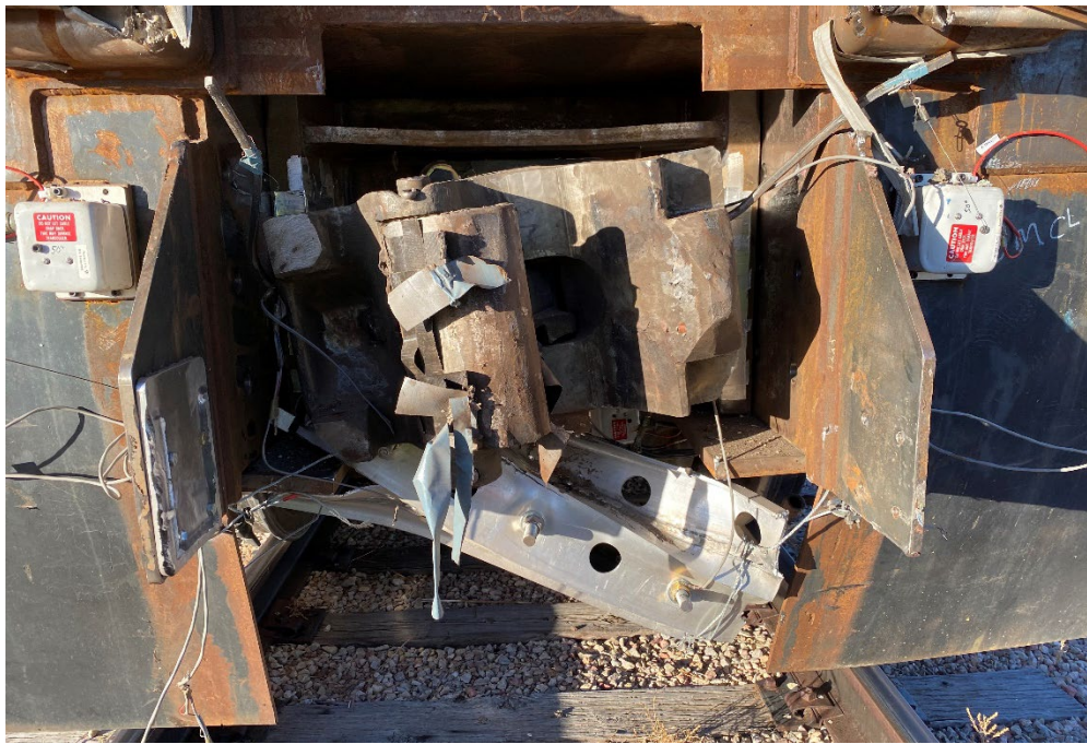
Figure 67. The deformed coupler carrier caught between the sliding lug and a bottom plate of the draft pocket
