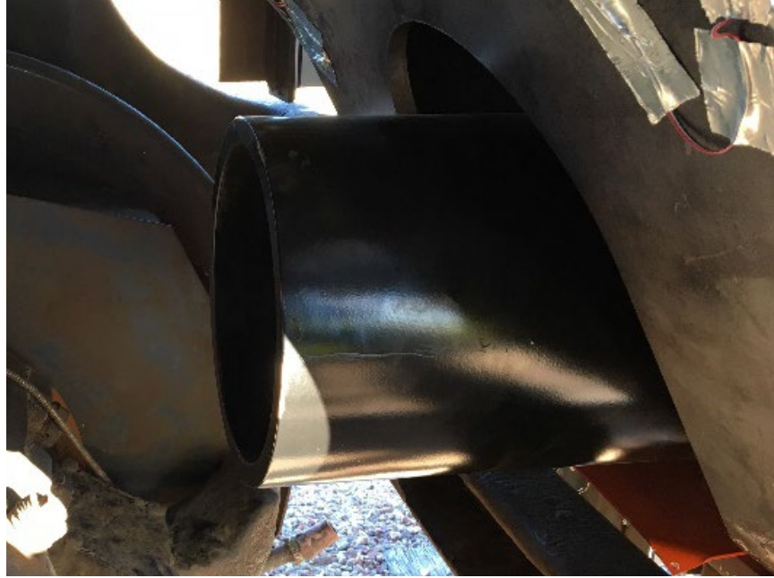
Figure 17. Pre-test photograph of the back of the PBC deformation tube
