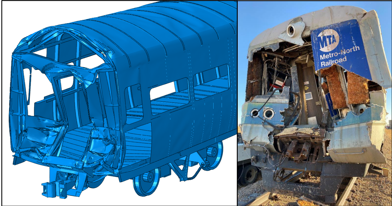
Figure 106. Comparison of FE model prediction (left) of cab car end frame mode of deformation with a post-test photograph of the end frame (right)
