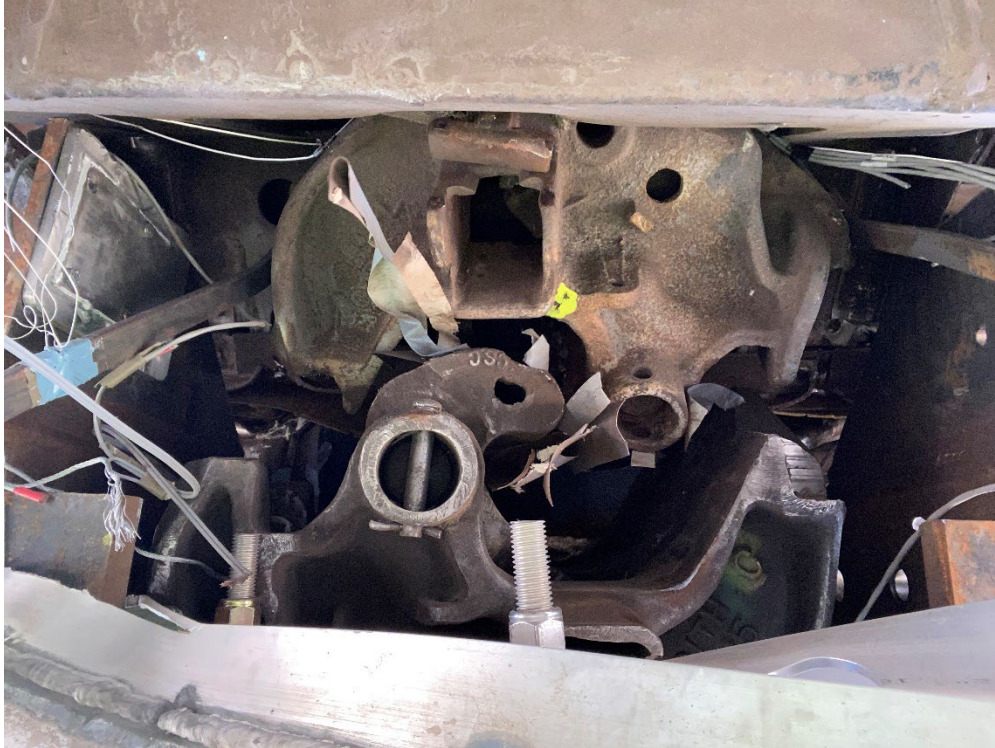
Figure 65. View of impacting couplers from below: M1 coupler on top, CEM loco coupler on bottom
