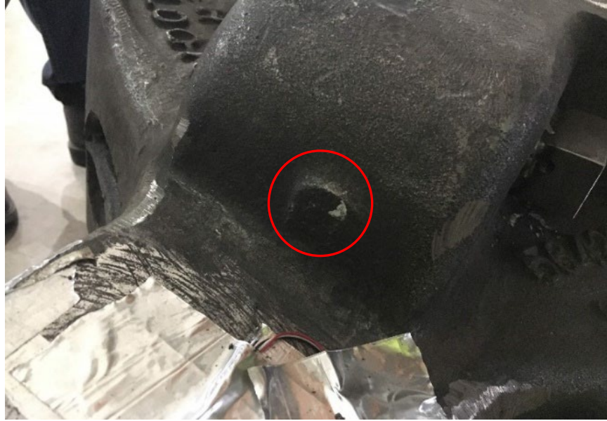
Figure 21. Damage to rear of the PBC coupler head from limit stop contact
