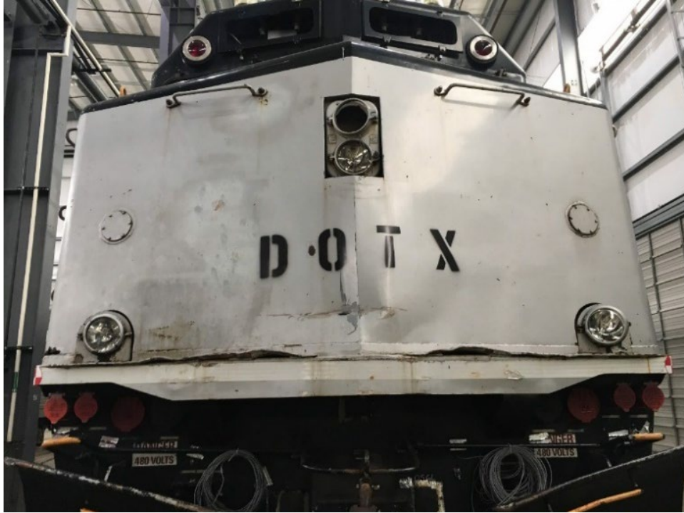
Figure 27. Conventional locomotive damage
