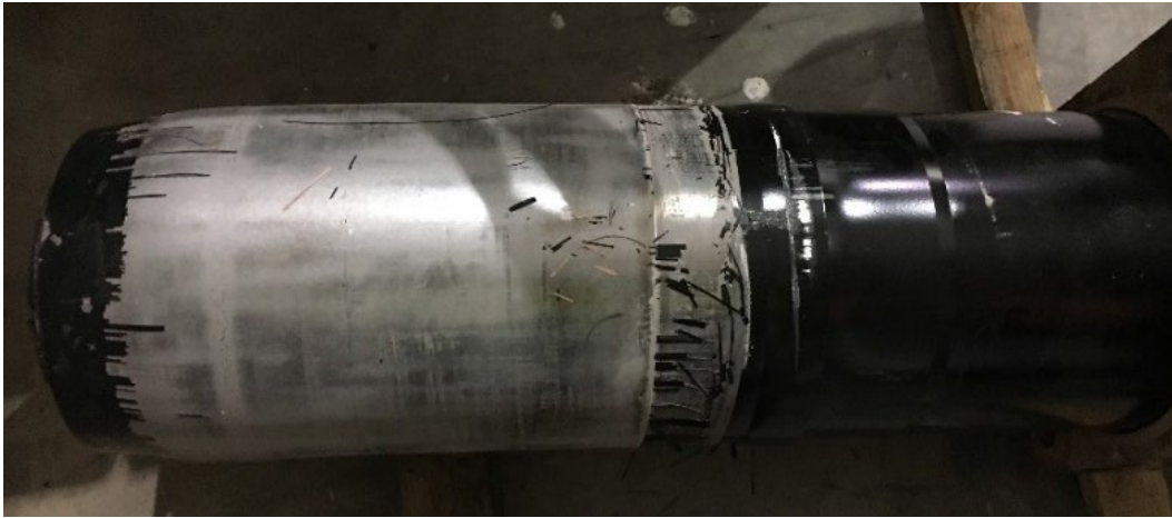
Figure 19. Deformed PBC deformation tube removed from the draft pocket; peeled paint has been removed
