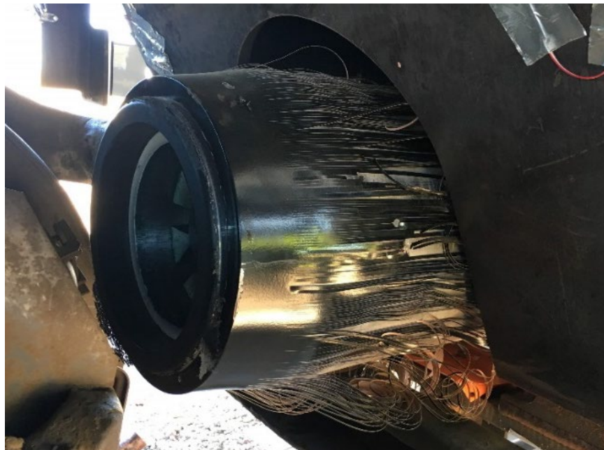
Figure 18. Post-test photograph showing the back of the PBC deformation tube
