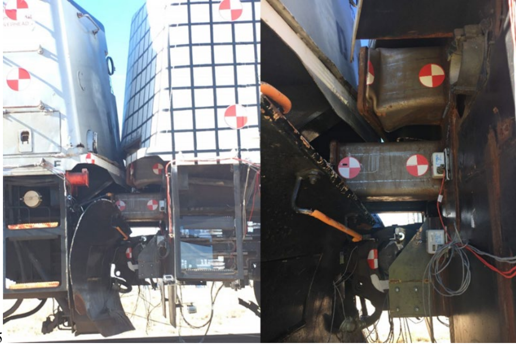
Figure 22. Post-test photo of CEM system; close-up on the right
