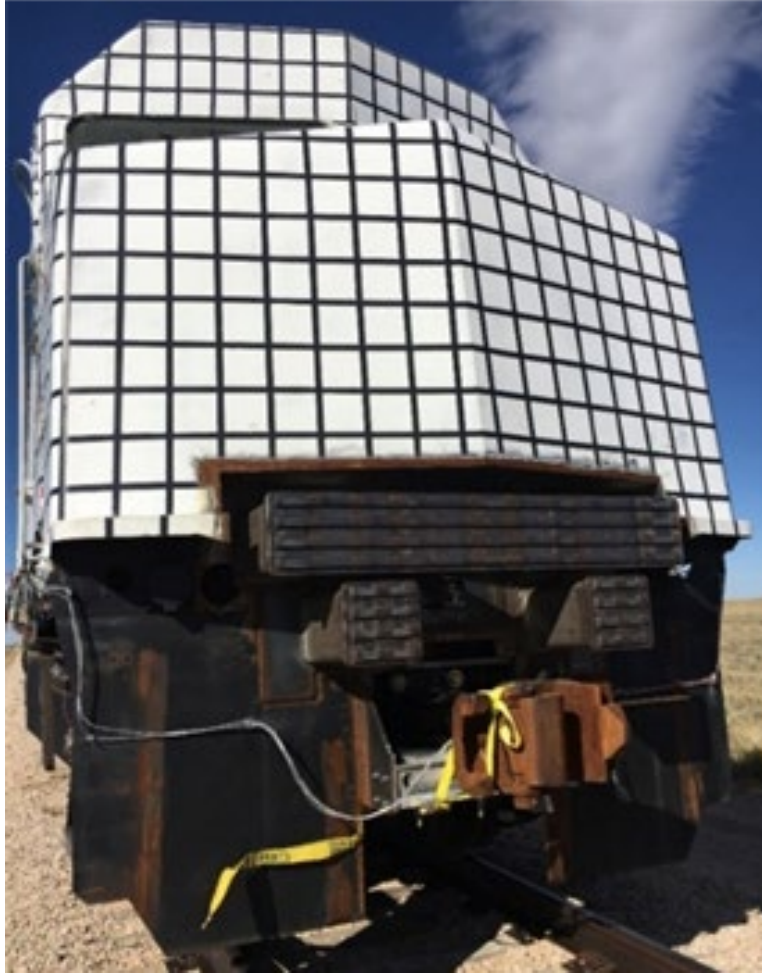
Figure 1. CEM locomotive comprising a DAC and PBC retrofit onto an F40 locomotive
