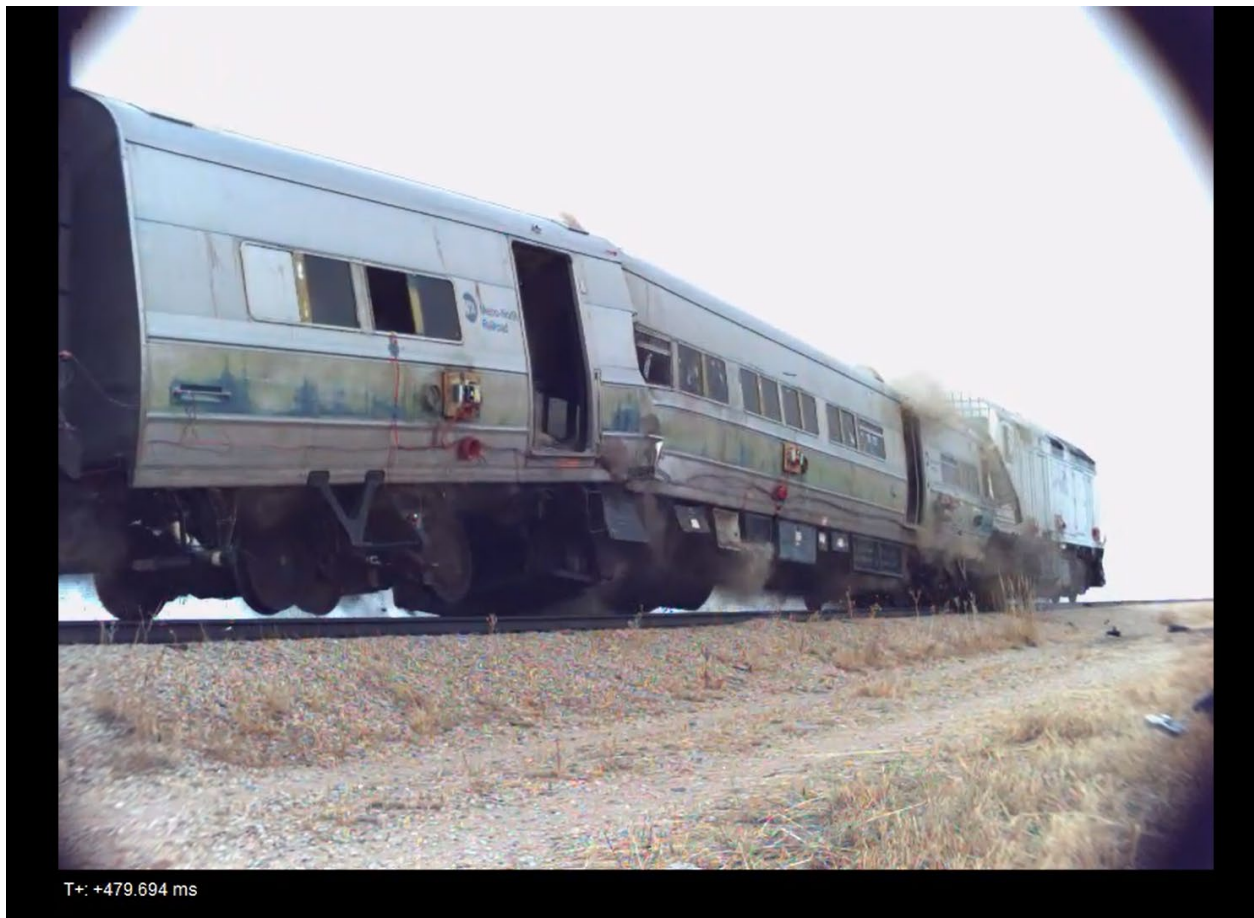
Figure 95. Image captured from high-speed video approximately 480 msec after impact, showing the upward folding of the cab carbody at the induced buckle just forward of the rear doors, causing the rear truck wheels to lift off the rail
