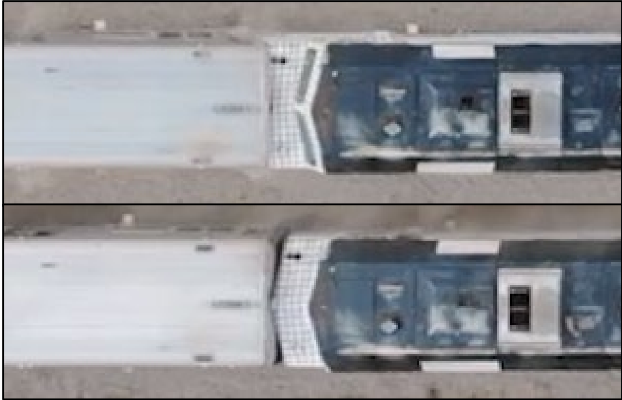
Figure 89. Still images from the overhead standing drone taken near the point of maximum crush (top) and after elastic rebound (bottom)
