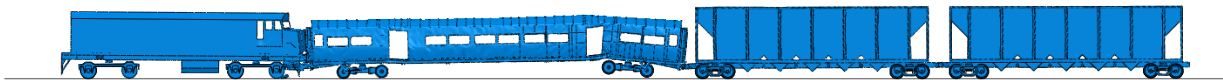
Figure 57. Predicted deformation after 0.25 seconds for a collision speed of 27.5 mph for model with flooring added back into the model, but only just past the forward door opening
