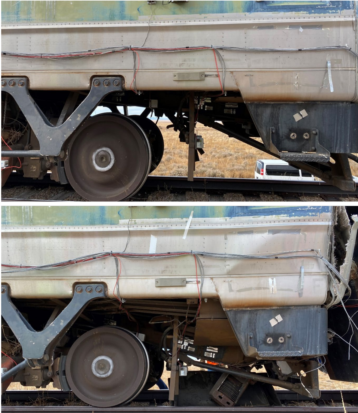
Figure 81. M1 draft sill before impact (top) and after impact (bottom)
