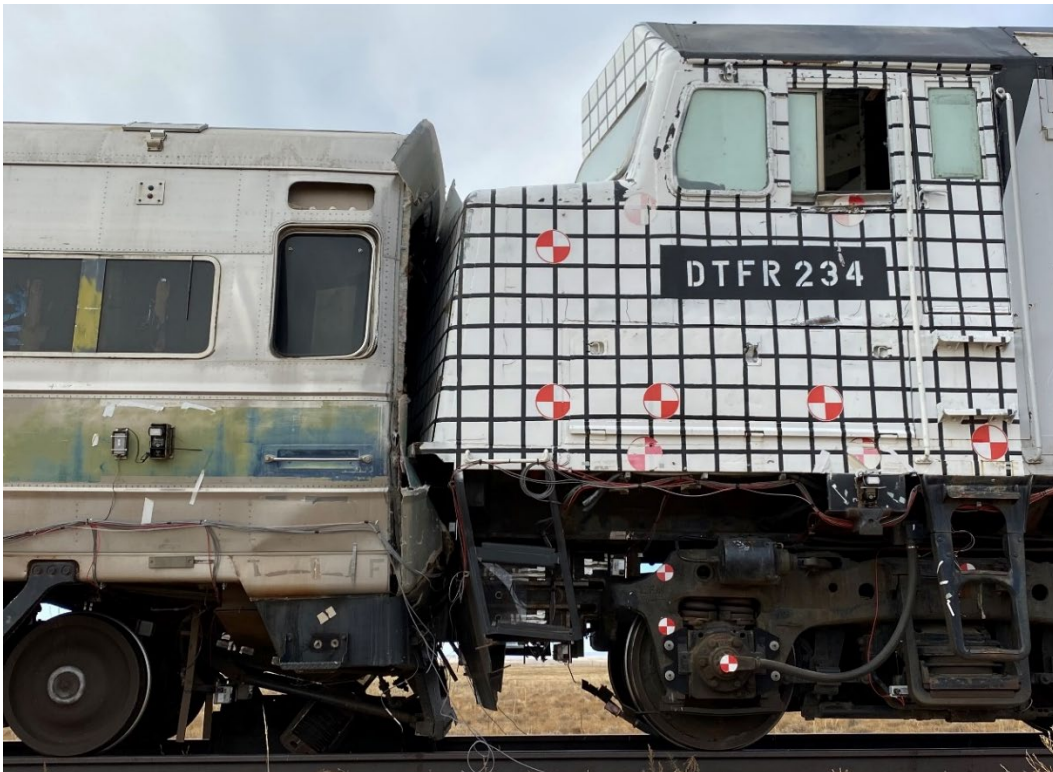
Figure 64. Post-test photo of the impact interface
