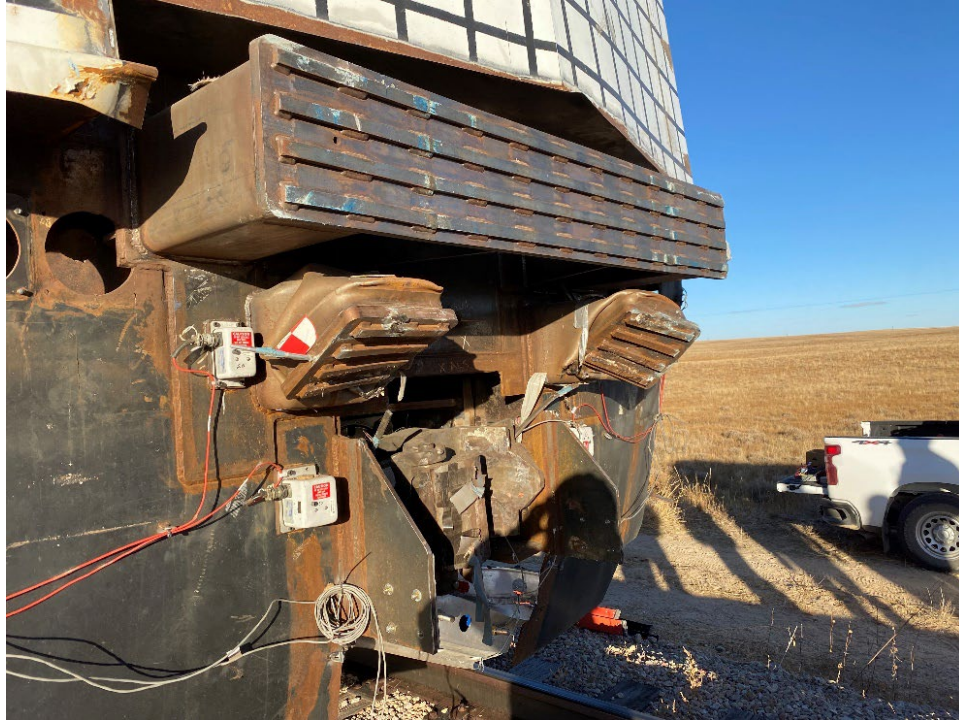
Figure 73. Upper and lower DAC tubes, post-test
