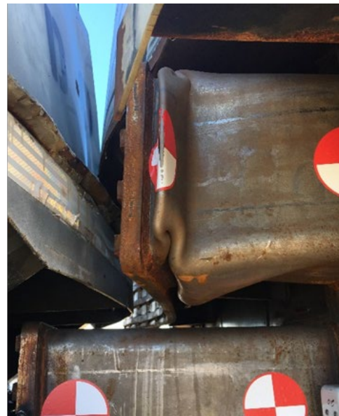
Figure 25. Deformed upper DAC tubes, right and left sides, respectively
