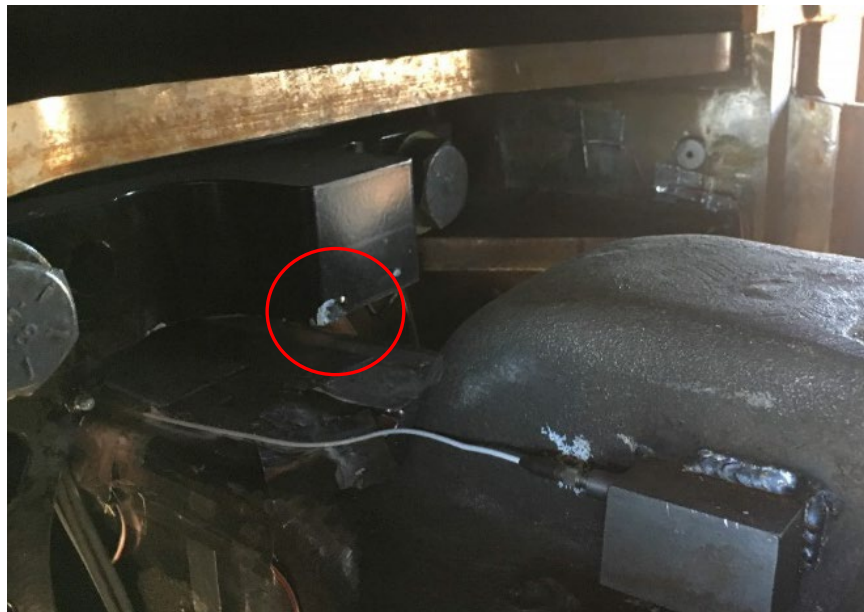
Figure 20. Damage to the limit stop mounted to the front of the sliding lug due to contact by the back of the PBC coupler head
