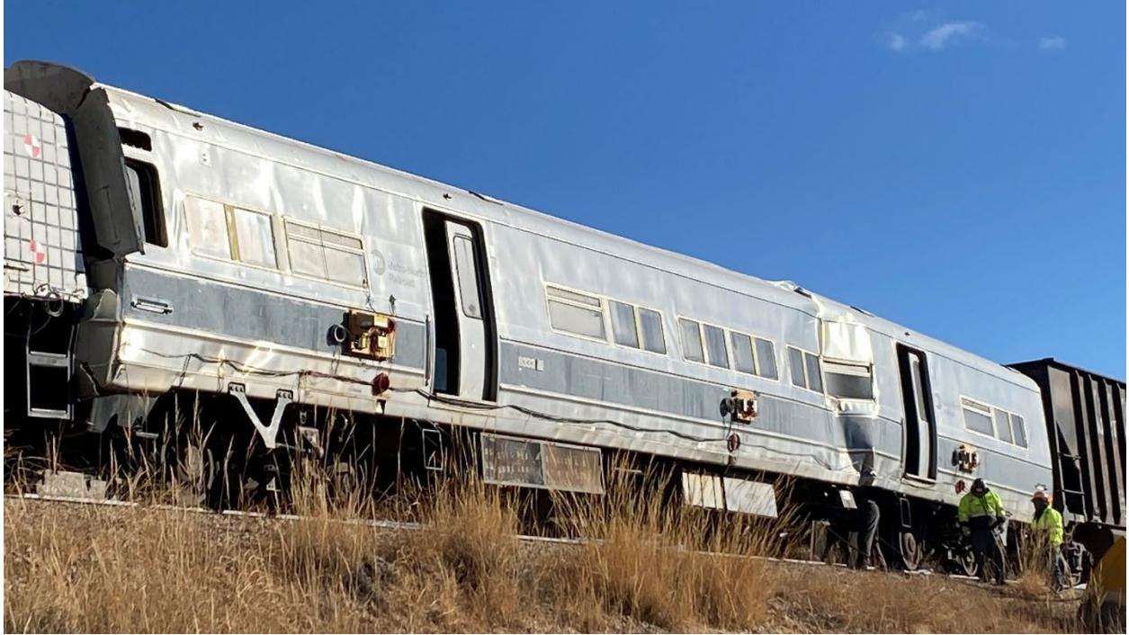
Figure 82. M1 carbody buckled inboard of rear doors
