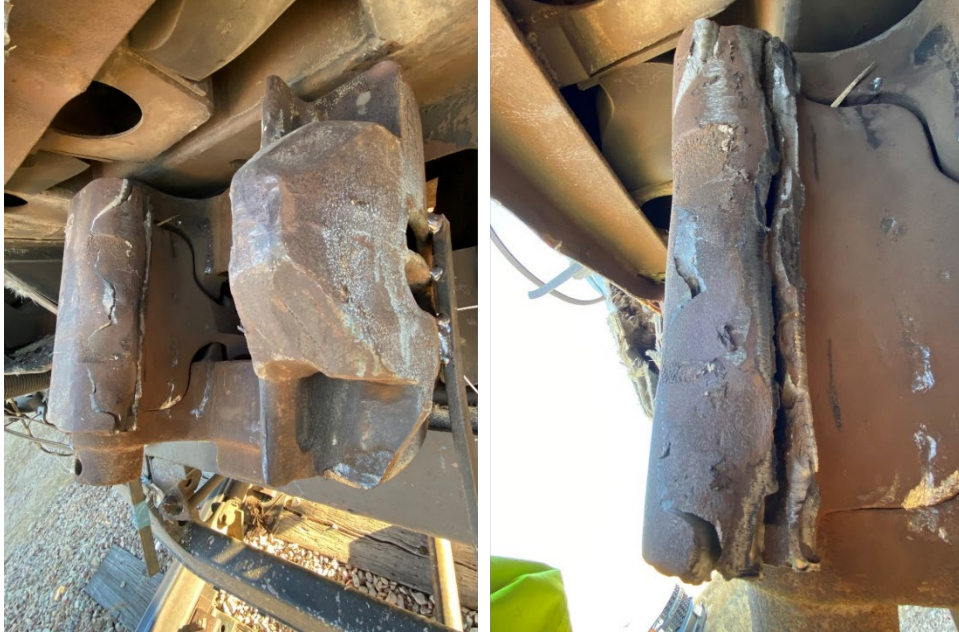
Figure 79. M1 coupler knuckle fracture (left), and a close-up of the fracture (right)
