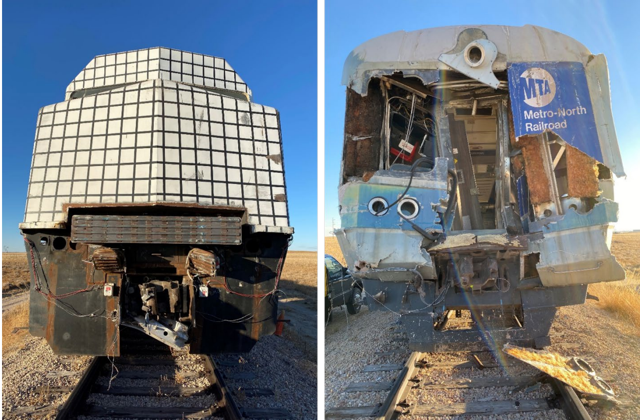
Figure 72. Post-test impact vehicles: CEM locomotive (left), M1 cab car (right)
