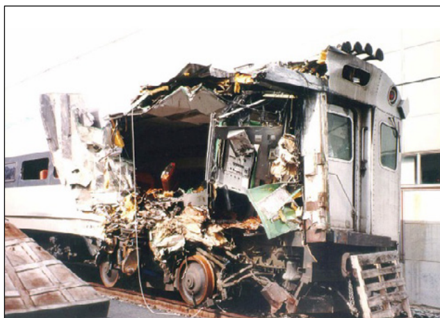
Figure 2-1 Decrease in occupant survival space and intrusion of external object 12
