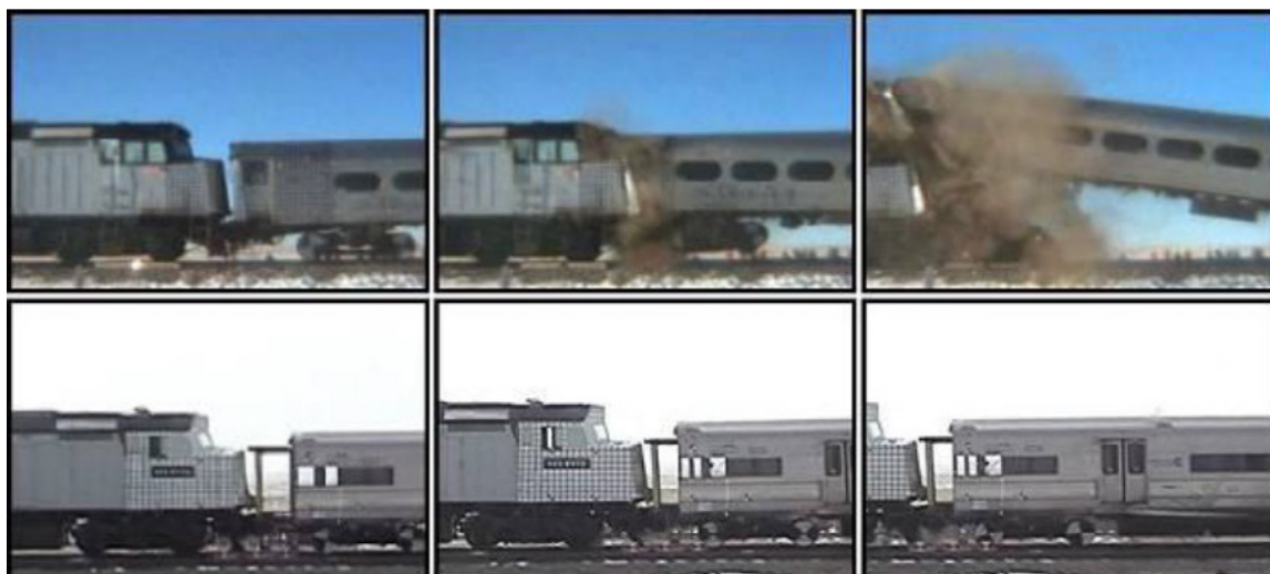
Figure 3-1 Conventional (top) and CEM-equipped (bottom) train-to-train crash tests 28
