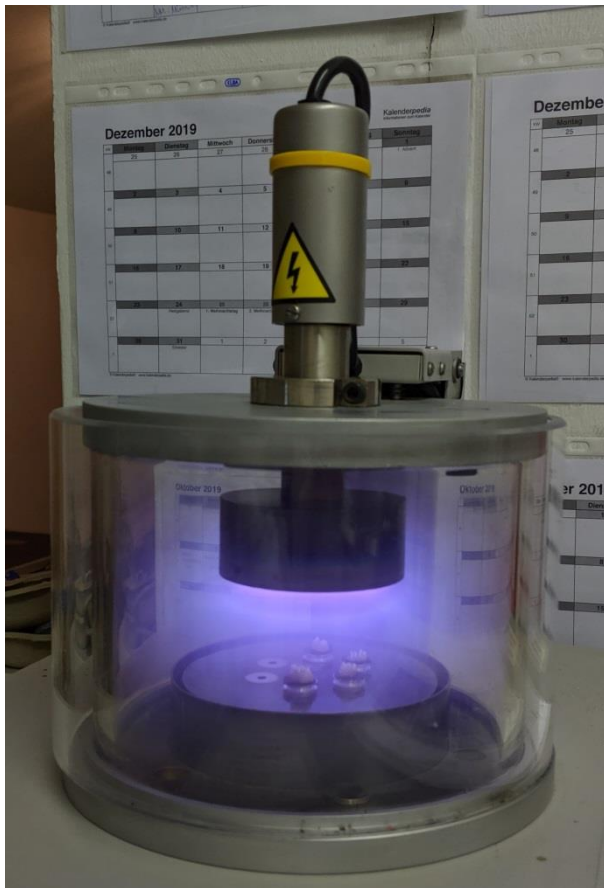
Abbildung 14: Sputter Coater, S150B, Firma Edwards
