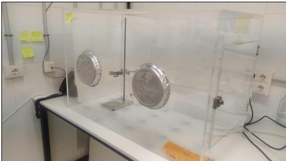
Figure 4: Empty glove box ready for use. Source: own elaboration.
