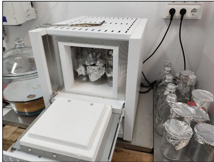
Figure 3: Nabertherm muffle furnace filled with material for sterilization. Source: own elaboration.
