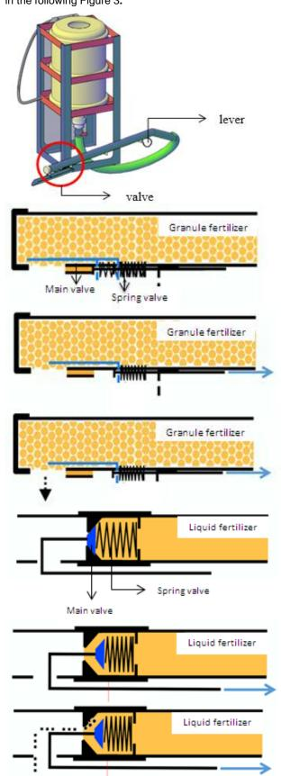
Figure 3. Work principles of a portable fertilizer device
