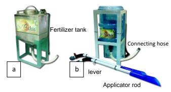
Figure 2. The Design of Fertilizer Devices (a) Type 1 and (b) Type 2
