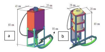
Figure 1. Design of Fertilizer Device (a) Type 1 and (b) Type 2
