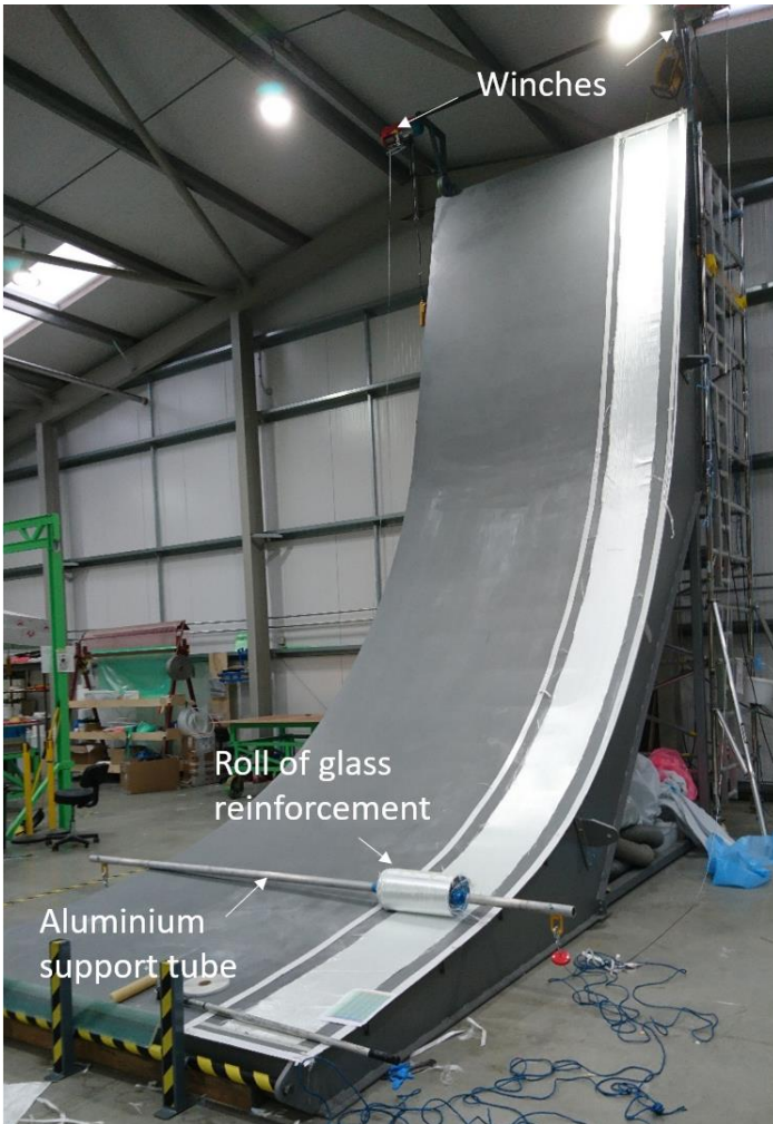
Figure 88: Testing material deposition tool during penultimate trial
