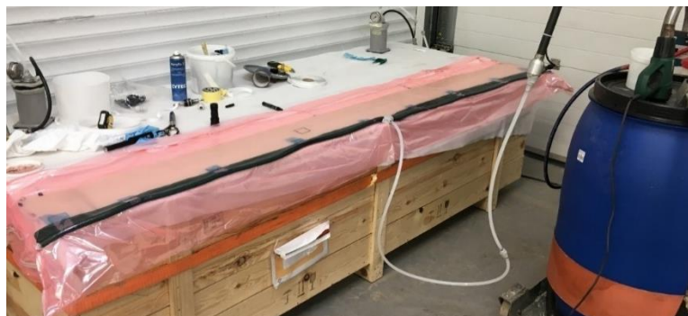
Figure 75: Wide infusion trial setup
