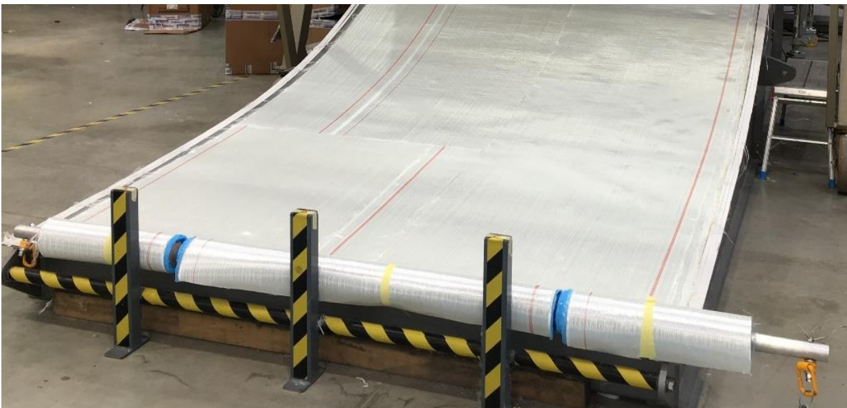
Figure 95: Layup of outer skin, showing ply staggering across the width and both short and medium plies
