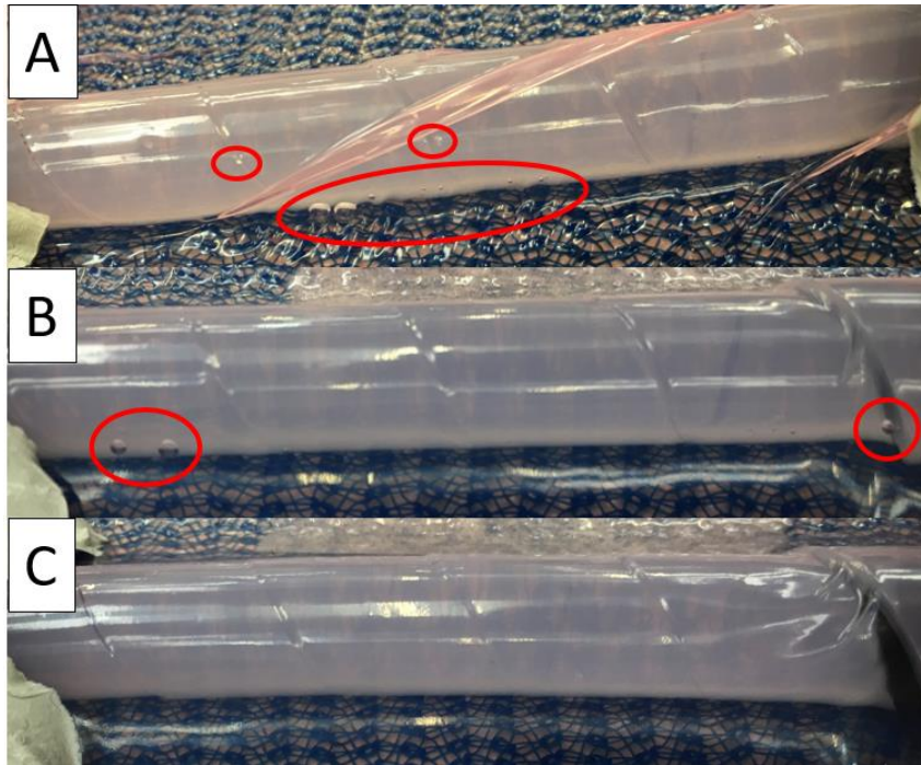
Figure 65: Bubbles (highlighted in red) within inlet spiral tube depending on time that resin was held at clamp. A = 0 minutes, B = 5 minutes, C = 60 minutes.
