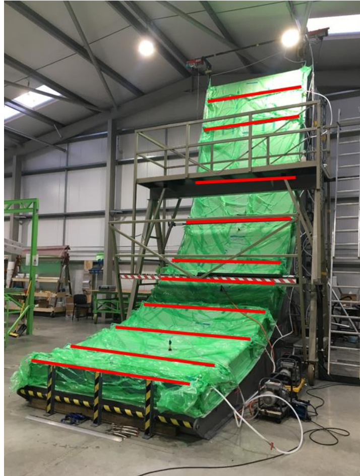
Figure 105: Demonstrator ready to infuse, resin inlets highlighted in red
