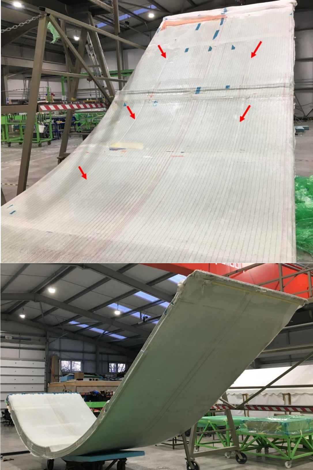
Figure 122: Demoulded Demonstrator. Top: Demonstrator inner skin (with grooves highlighted), Bottom: Outer skin
