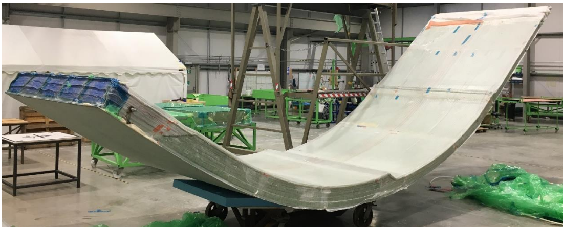
Figure 115: Cured and demoulded demonstrator
