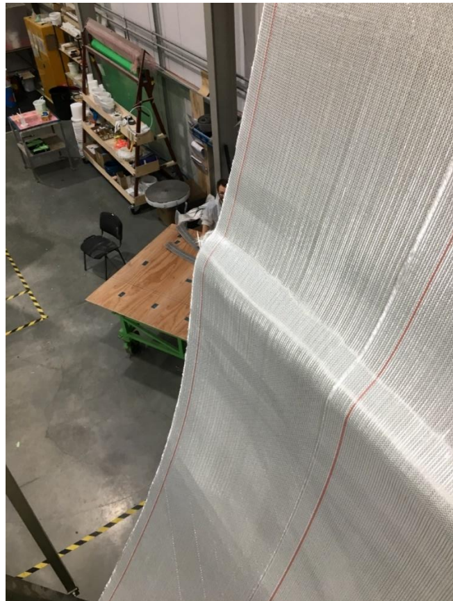
Figure 103: Potential for fibre bridging within the inner skin across joint 2 transition
