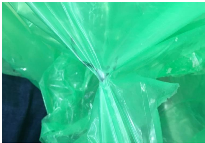
Figure 116: Inner and outer vacuum bags welded together (photo taken after demoulding to highlight welding effect)
