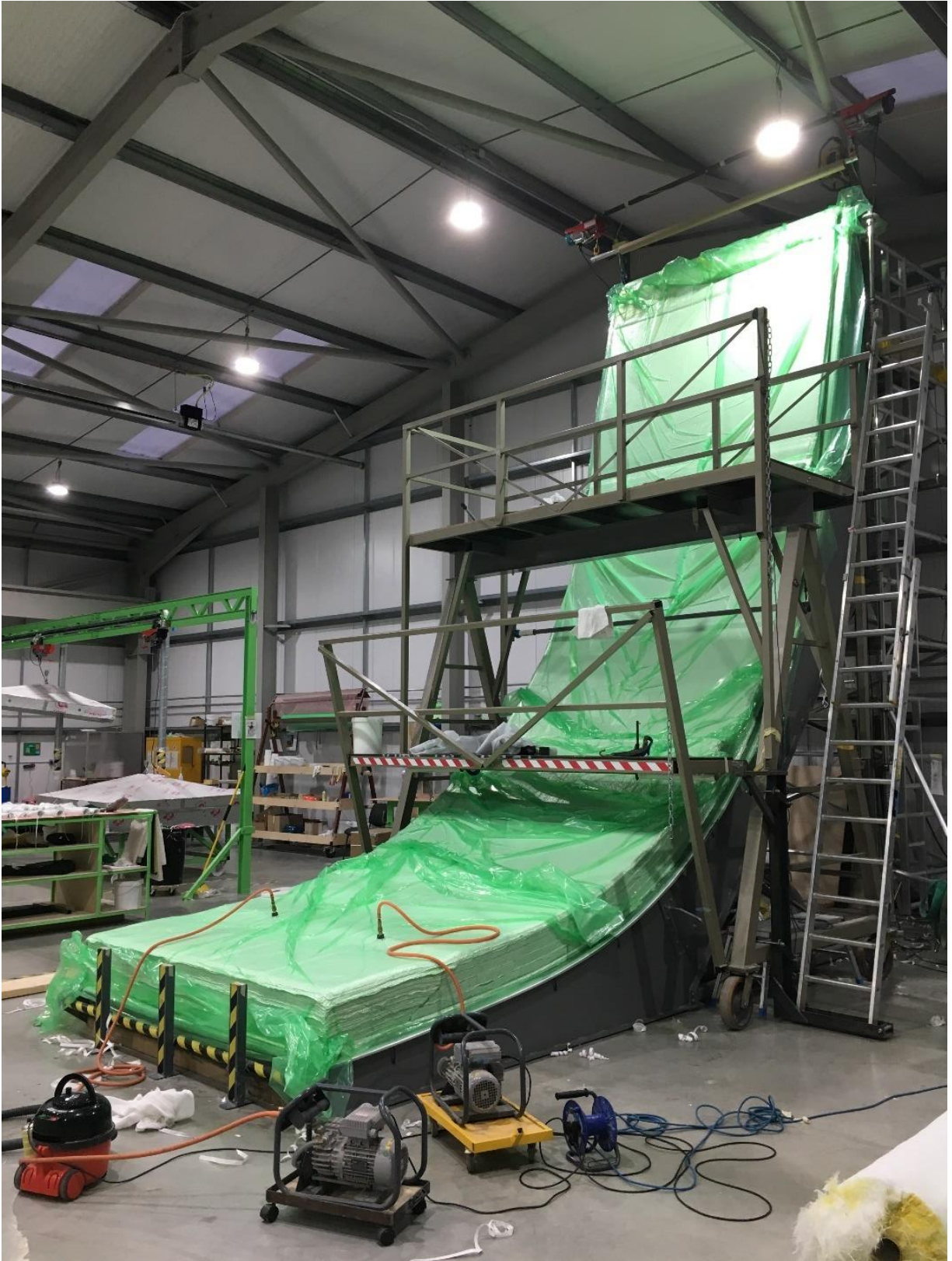
Figure 104: Completed demonstrator layup under vacuum
