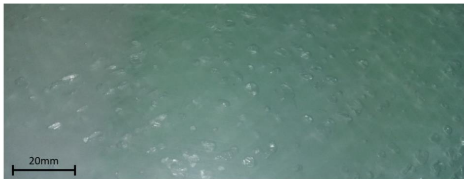
Figure 63: Evenly dispersed voidage within a large cured composite section
