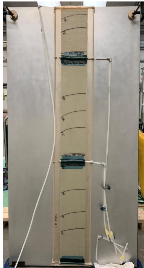
Figure 41: Vertical infusion on aluminium tool surface
