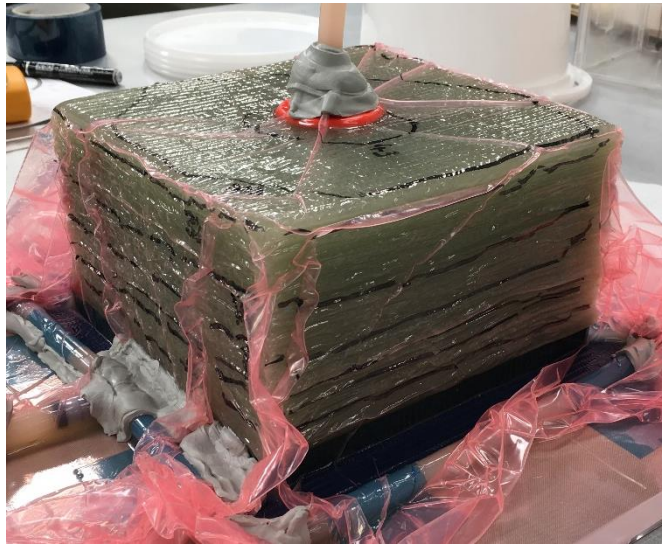
Figure 59: Monolithic block laminate infused through-thickness
