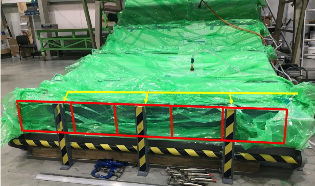
Figure 106: Monolithic keel resin inlet. Spiral tube network (red) and resin delivery tubes (yellow)
