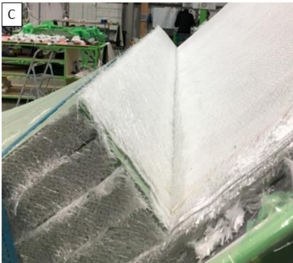
Figure 99: From top to bottom right: Infusion of joint 1 support, Positioning joint 1 support on tool, Two plies of Saefflow on top edge of SP1, Joint 1 support positioned between SP1 and SP2.
