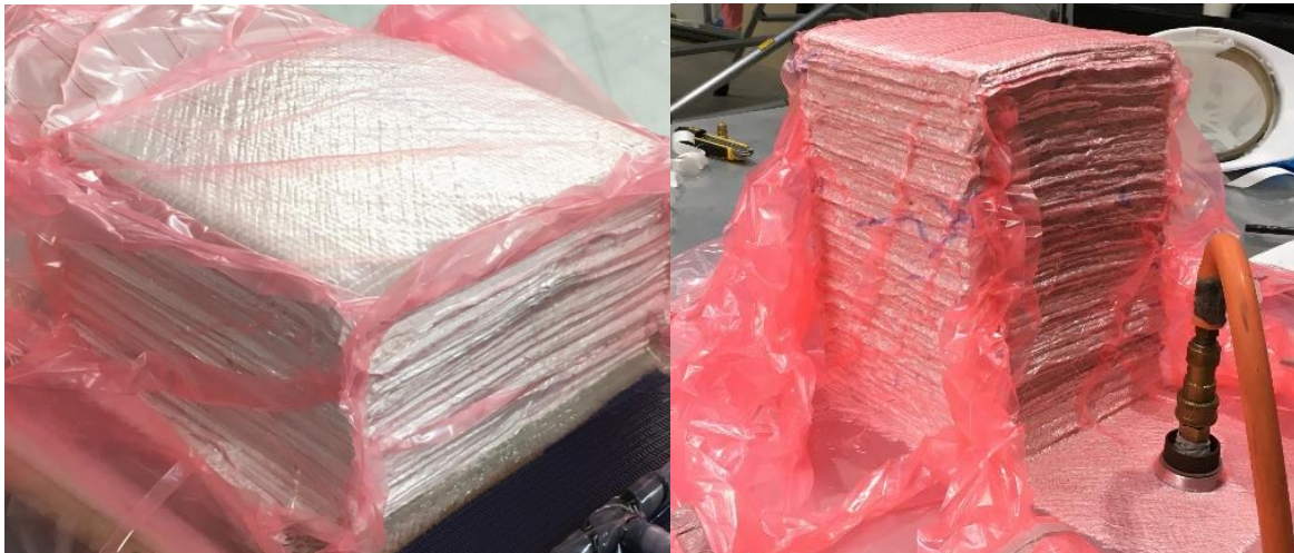
Figure 21: Thick monolithic laminate debulk investigation
