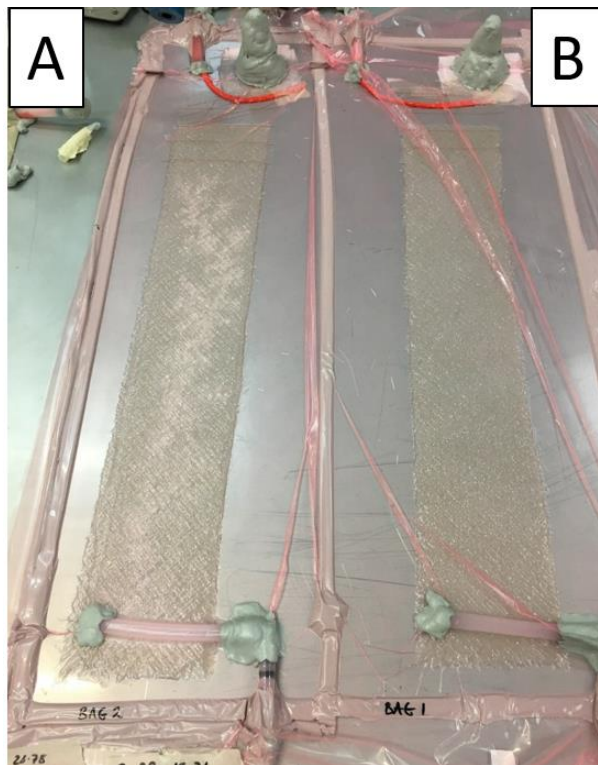
Figure 69: Laminate infusions with a fibre bundle (A) and single fibre (B) crossing tacky tape seal
