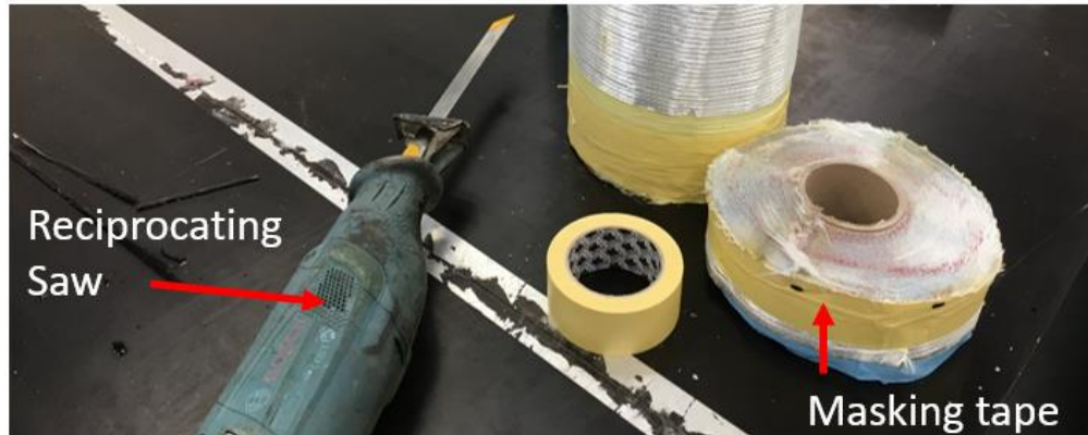
Figure 90: First attempt at cutting glass reinforcement rolls
