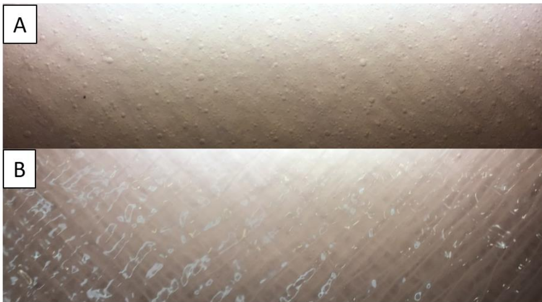
Figure 76: Bubbles within laminates immediately after infusion. A: Current degassing procedure, B: New degassing procedure (concept 5).
