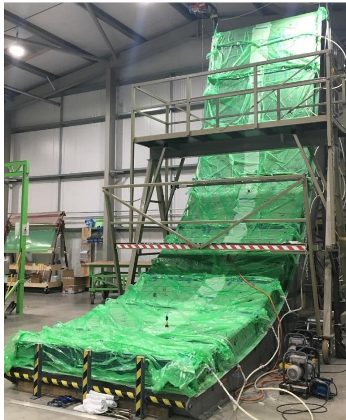
Figure 109: Fully infused demonstrator (white strip in centre is bleeder fabric between inner and outer bags)
