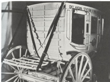
View showing the luggage rack at the back of the Stagecoach body.
