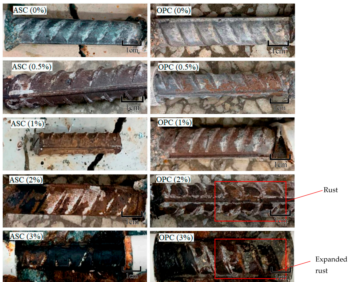
Figure 3. Steel bar corrosion in ASC and OPC at different designed corrosion degrees.
