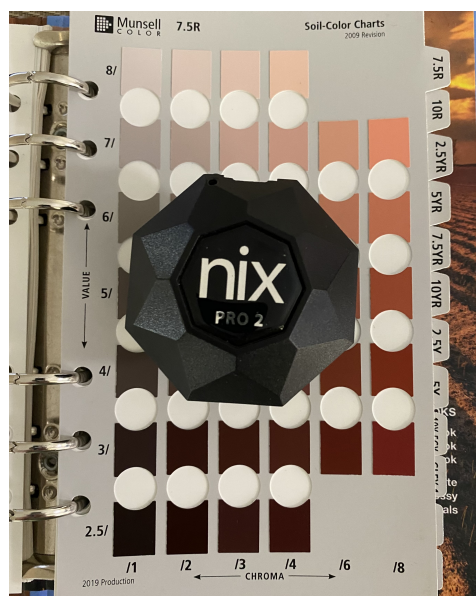
Figure 4. Data collection of ground-truth data using Nix Pro.
