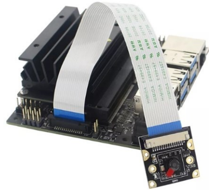
Fig. 5. Jetson nano with 8MP Sony IMX219 77-degree CSI camera
