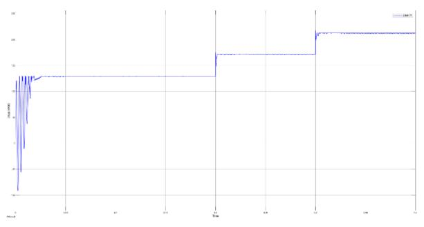
Fig. 6. Power change of solar photovoltaic with change of solar irradiance at 25  $^{\circ}$ C
