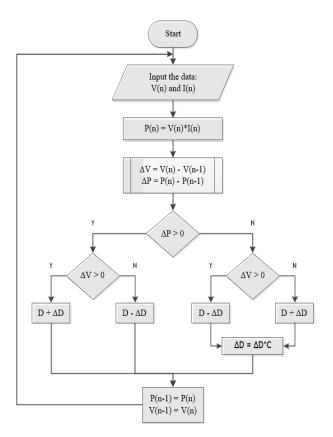
Fig. 3. Flowchart of the modified Perturb and Observe (PO) algorithm [6]
