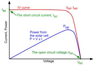
Fig. 1. Current voltage (IV) curve of a solar cell [26]. Operation at the point of maximum power is required to get the maximum power output of the solar cell.
