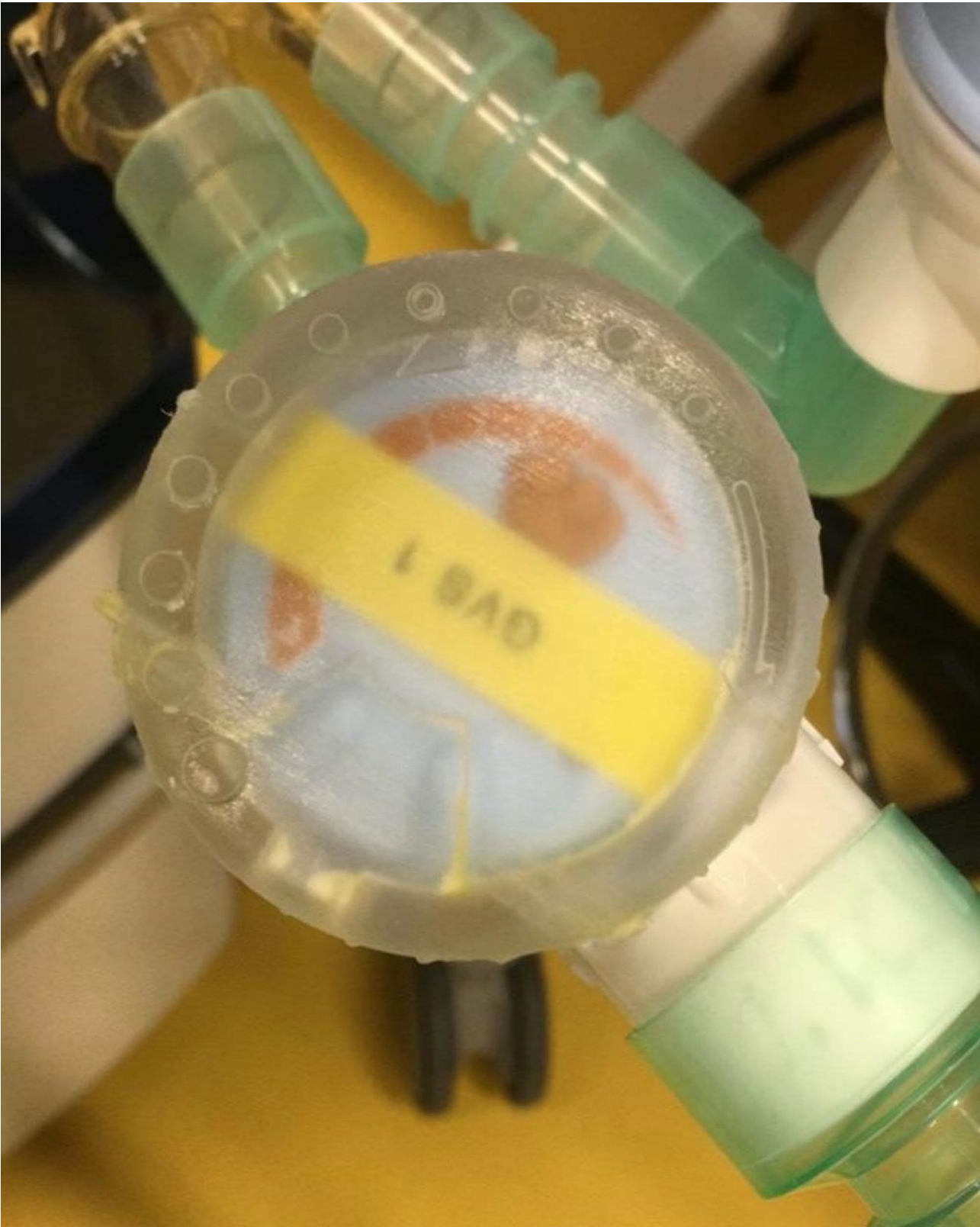
Fig. 3 Photograph of control cap custom designed and applied to the top of the APL valves to allow more precise control and testing of the shared circuit
