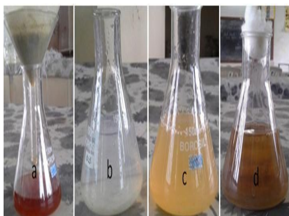
Fig. 2. Visual appearances of flask containing the aqueous extract of A. malabarica leaf and AgNO 3 solution after 48h reaction time a) Aqueous extract of Anisomeles malabarica leaves. b) 1mM AgNO 3 . c) Reaction mixture 0 min incubation. d) Reaction mixture after 48h incubation at room temperature.
