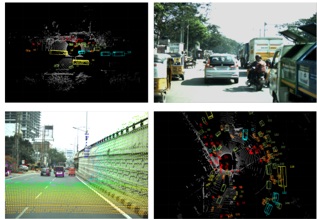
Figure 1. Some examples from the dataset showing different traffic scenarios, LiDAR data with annotations, and a sample of LiDAR point clouds projected on camera data.
