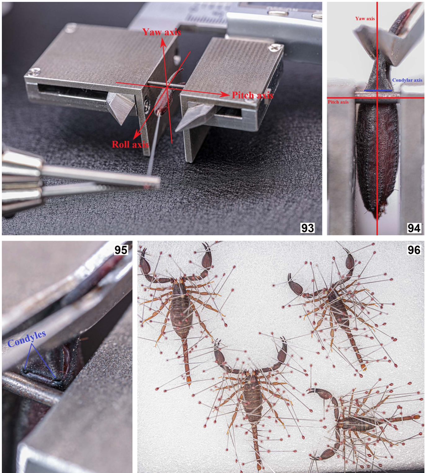
Figures 93–96. Application of “condyle method” upon a modified caliper (93–95) using the right chela of an adult male S. xui as the example, and pinned specimens of S. tongtongi (96). In reality, to avoid the deviation caused by the curvature of chelal fingers, the chela needs to be positioned in a vertical direction (Fig. 94); this obviously depends on the width of the L-shaped plate. The chela does not have to be orthogonal to a horizontal plane since the rotation around the pitch axis does not affect the width measured, as long as the roll and yaw axes are fixed (thus defining a 2D plane) based on the rod (however, this could be difficult by manual measurement).
