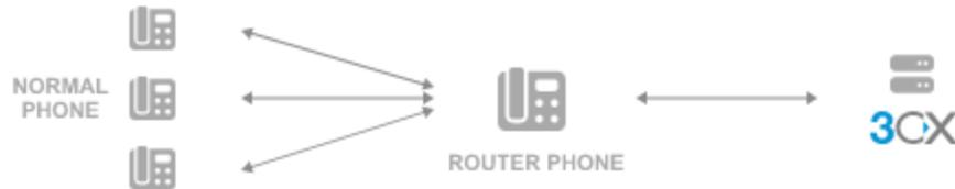
In a hosted / public cloud environment all voice traffic must be proxied via a router phone or an SBC. If you do not have an SBC or router phone already, your first phone must be a router phone. Select the type of IP Phone to add:
