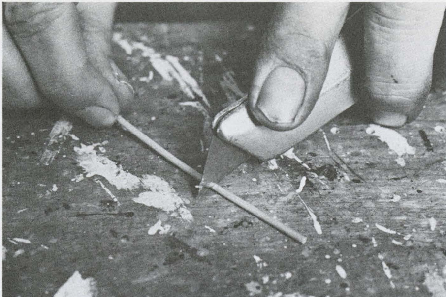
Cutting the masts.
