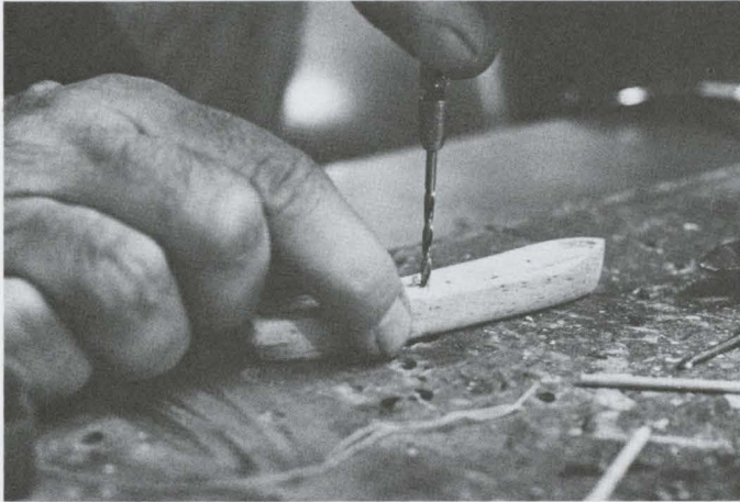
Drilling three holes for the masts.
