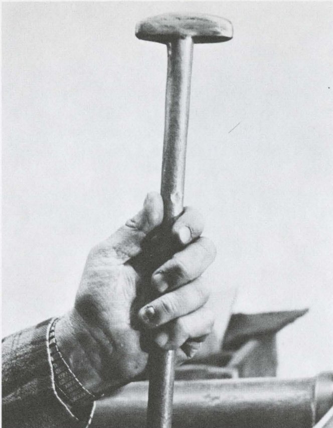
The setting bottom tool is used in smoothing out the bottom of the bowl.
