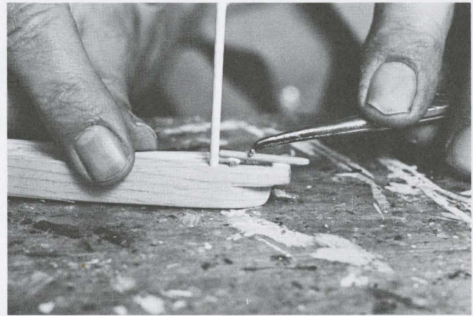
Gluing the boom onto the boom rest.
